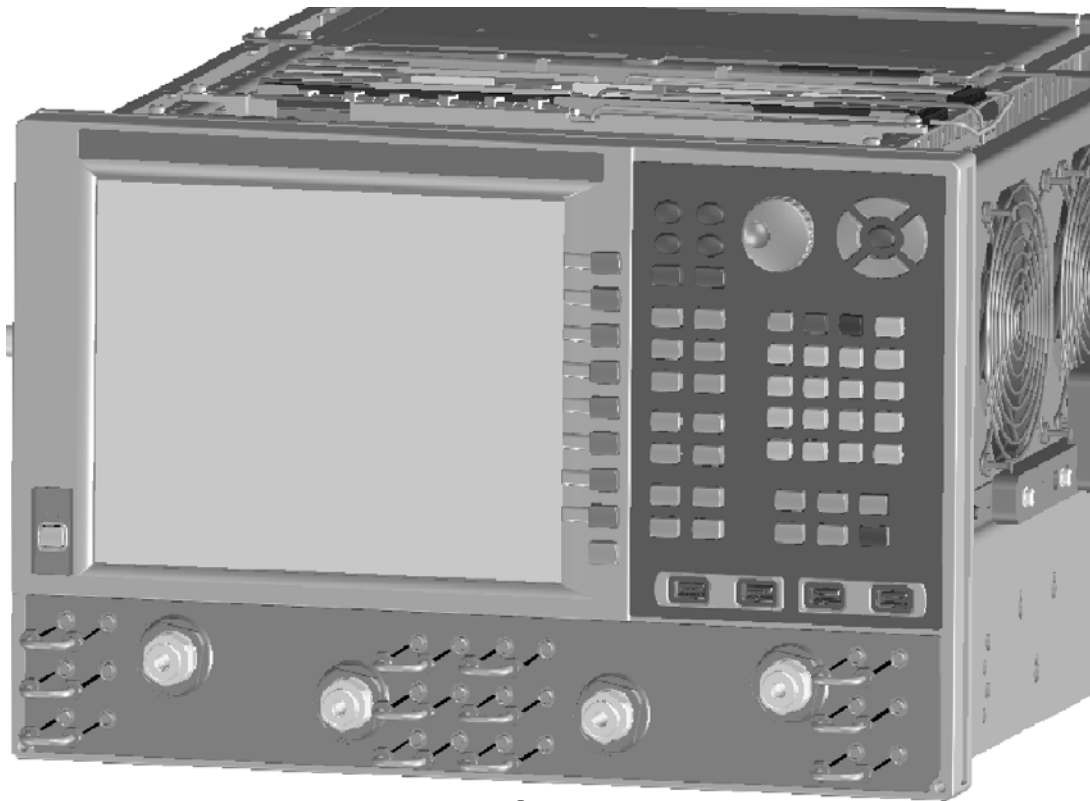
Figure 8 Front Panel Jumper Cables Installation
