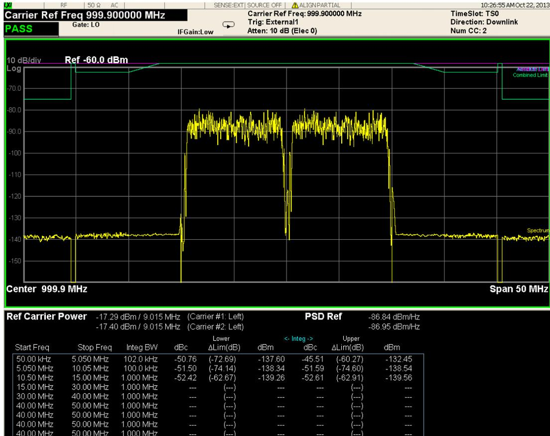
For WLAN 802.11ac (80 + 80 MHz), power readouts of both of the carriers are displayed in the lower result window.
