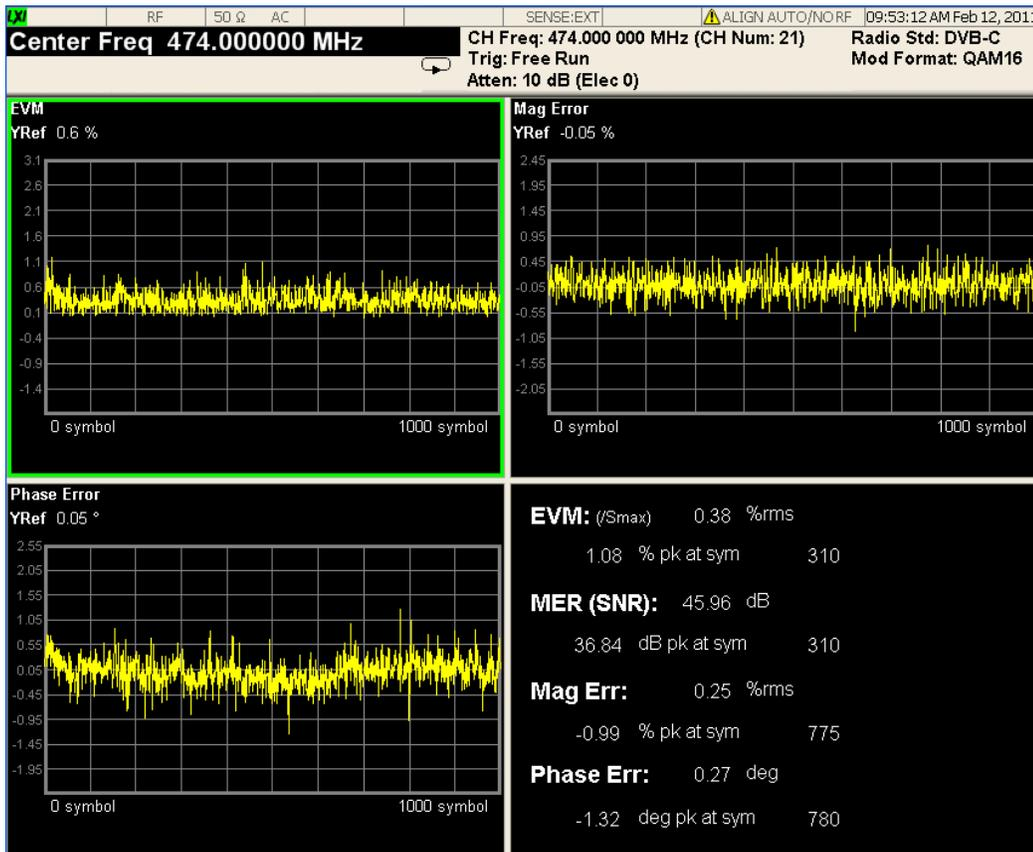
Figure 5 – 17 I/Q Error View of Modulation Accuracy Measurement (Scale Type is EVM)
