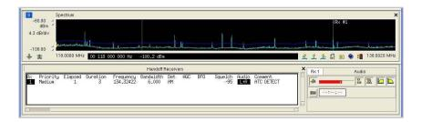
With Keysight's N6829BS "Snapshot Radio Player", a user can playback IQ recordings and demodulate using AM, FM, USB, LSB, and CW. Voice inversion is also possible. Snapshot Radio is sold separately from Surveyor 4D, but is a great companion product for those processing large amounts of audio files.
