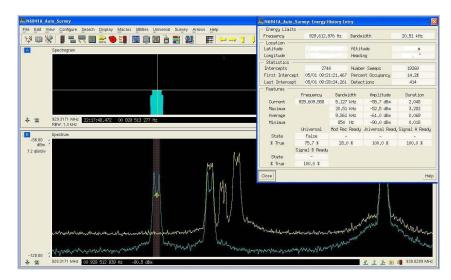
The EHD is used as an interim repository where intercept data is further processed and refined through Energy History Filtering and Alarms.
