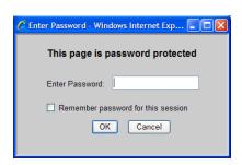
By default, this password is set at the factory as "agilent". However, you may subsequently change the password. (Press **System**, **I/O** Config, **Reset Web Password** on the instrument front panel to change the password.)
