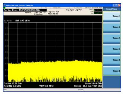
If a displayed key label shows a small solid-black arrow tip pointing to the right, it indicates that additional key menus are available. If the arrow tip is not filled in solid then pressing the key the first time selects that function. Now the arrow is solid and pressing it again brings up an additional menu of settings.
