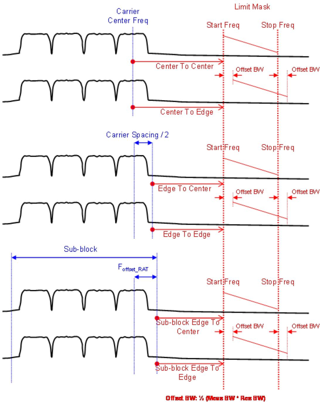
Offset Freq Definition (Limit Mask) in SEM measurement
