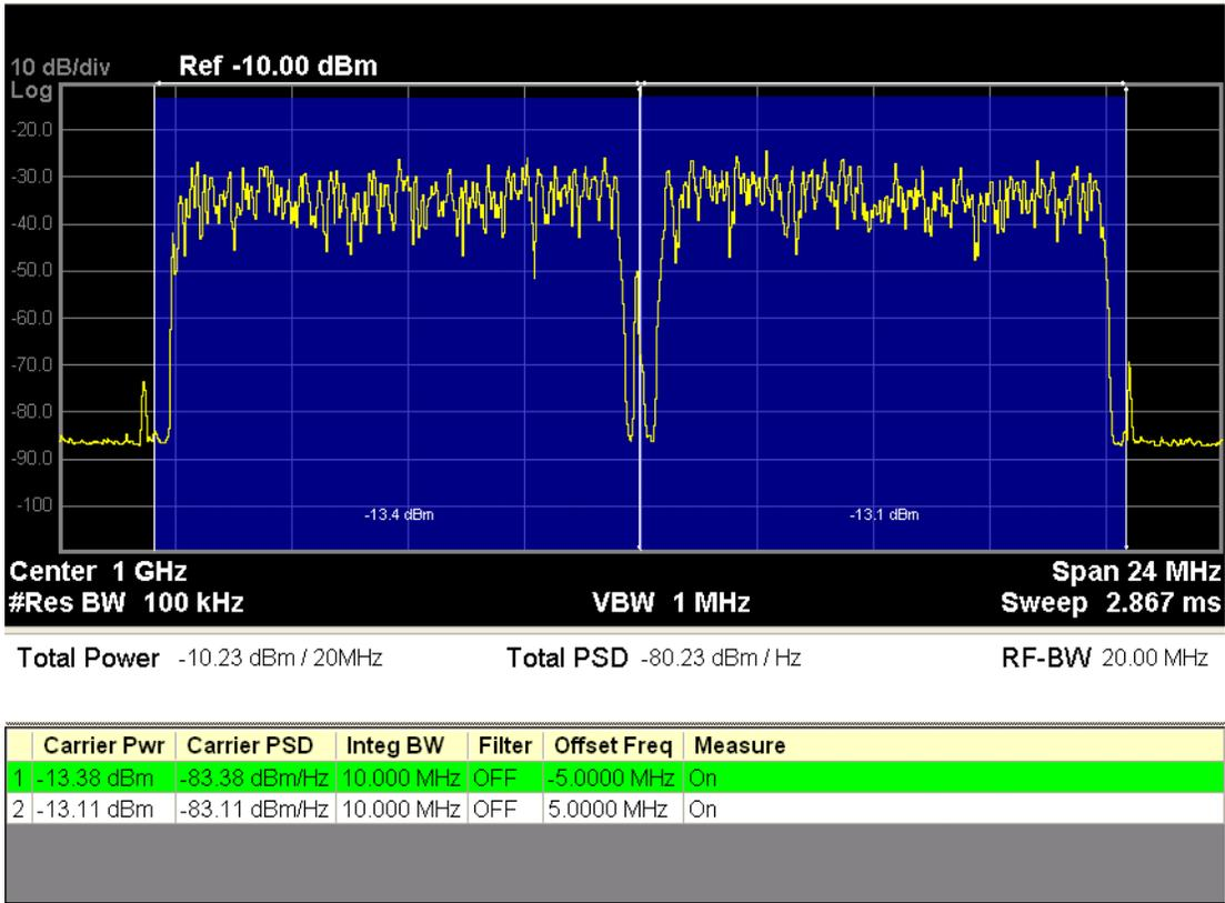
Figure 0-9 Carrier Info view of LTE-Advanced FDD/TDD CHP
