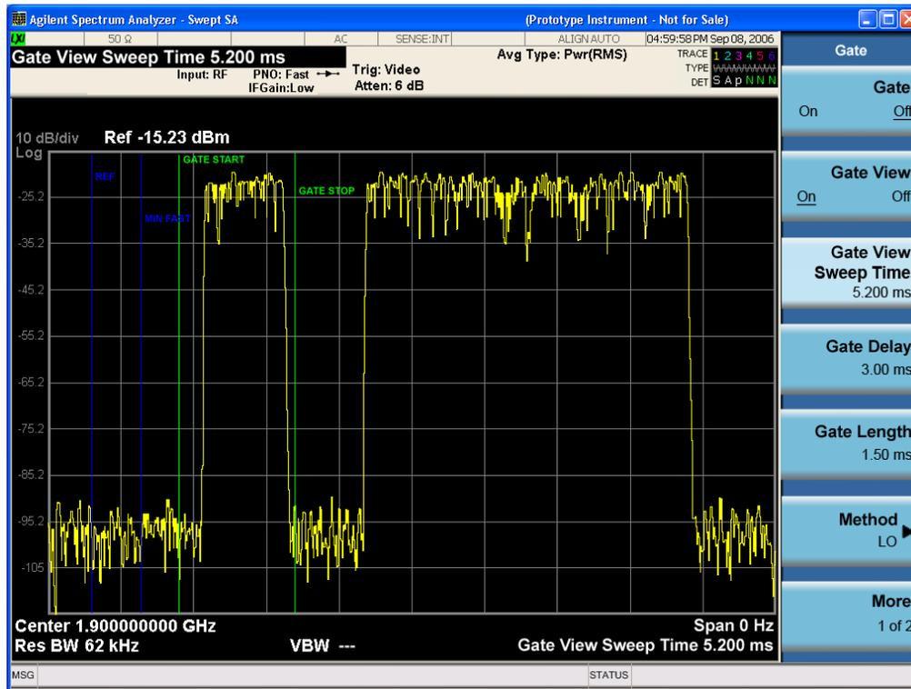
A sample of the Gate View screen in other measurements is shown in the following graphic . This example is for the ACP measurement:
