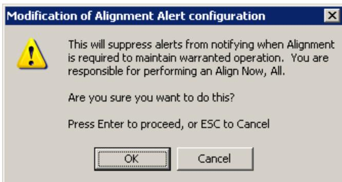
No confirmation is required when Alert is configured through a remote command.
