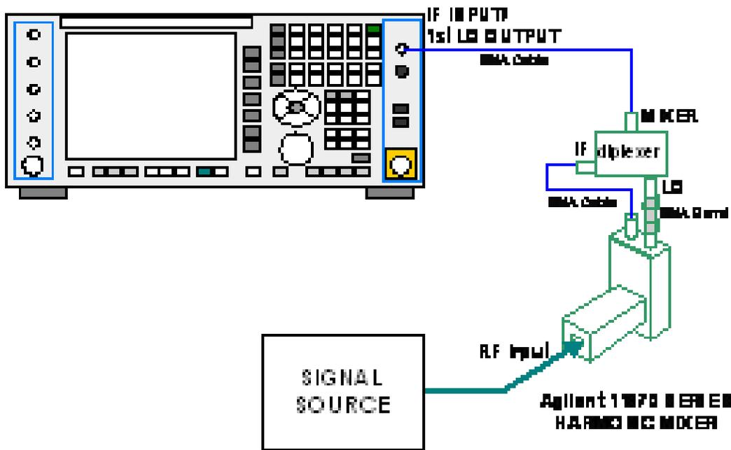
In addition, External Mixing in the X-Series supports the new Agilent M1970 series of Harmonic Mixers, which provide a USB connection for download of calibration data and additional control.
