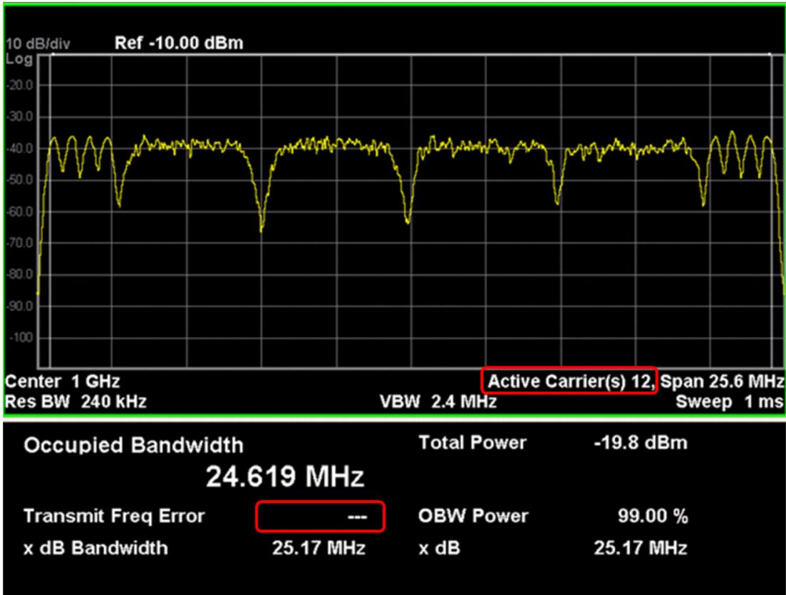
The number of active carriers is displayed. Since span is determined from detected carriers in auto mode, it is necessary to show how many carriers are identified as active., as highlighted above.
