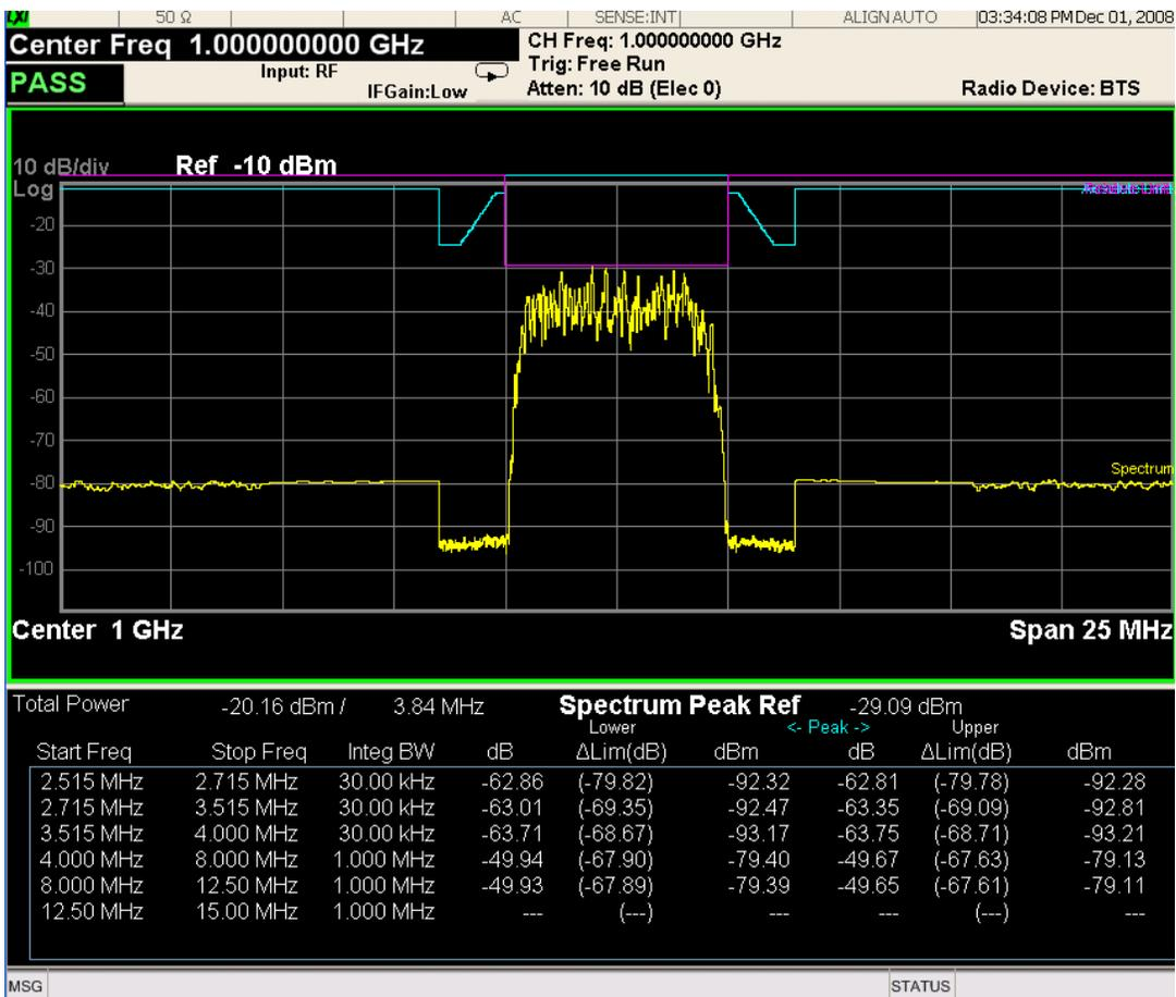
For WLAN 802.11 ac (80 + 80 MHz), power readouts of both of the carriers are displayed in the lower result window.
