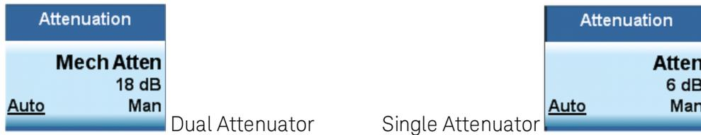
In the single attenuator configuration, you control the attenuation with a single control, as the fixed stage has only two states. In the dual attenuator configuration, both stages have significant range so you are given separate control of the mechanical and electronic attenuator stages.
