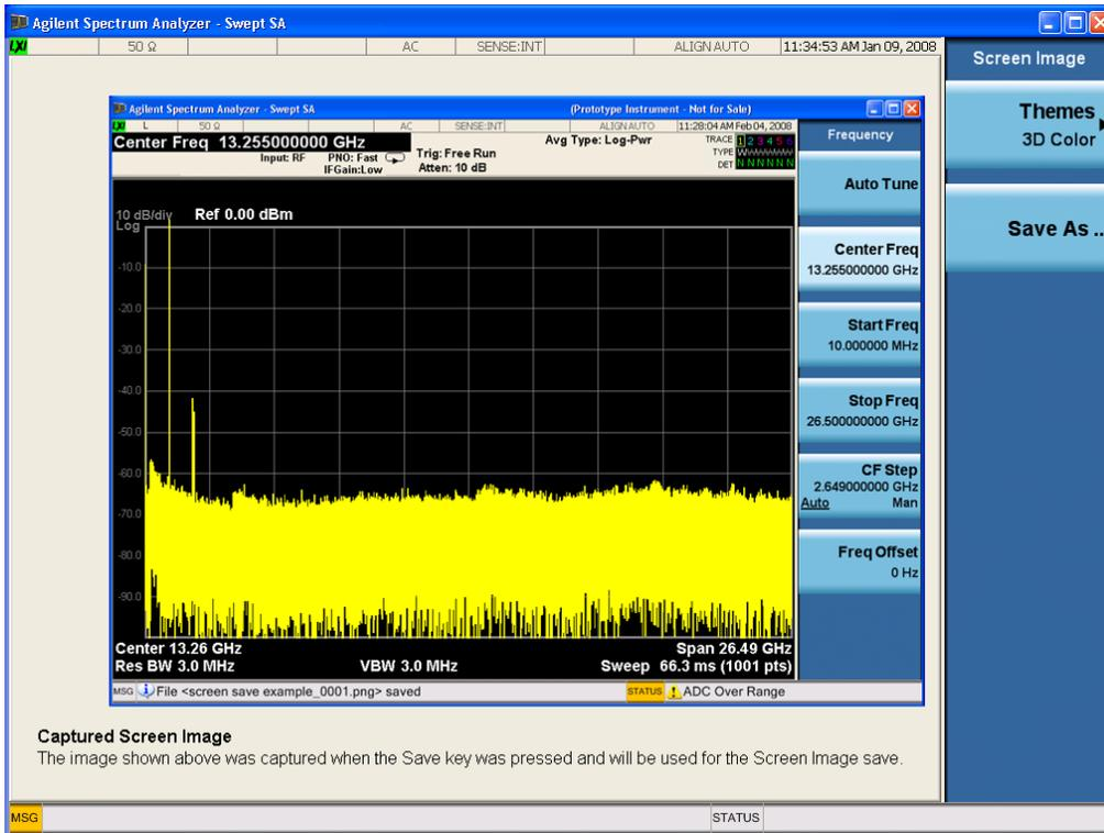
When you continue on into the Save As menu and complete the Screen Image save, the image depicted in the thumbnail is the one that gets saved, showing the menus that were on the screen before going into the Save menu. The save is performed immediately and does not wait until the measurement is complete.
