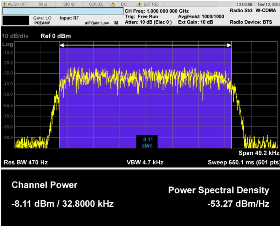
If current mode is MSR and LTE-Advanced FDD/TDD, there are two views, Power Results and Carrier Info. Power Results view is almost the same as the common CHP view.
