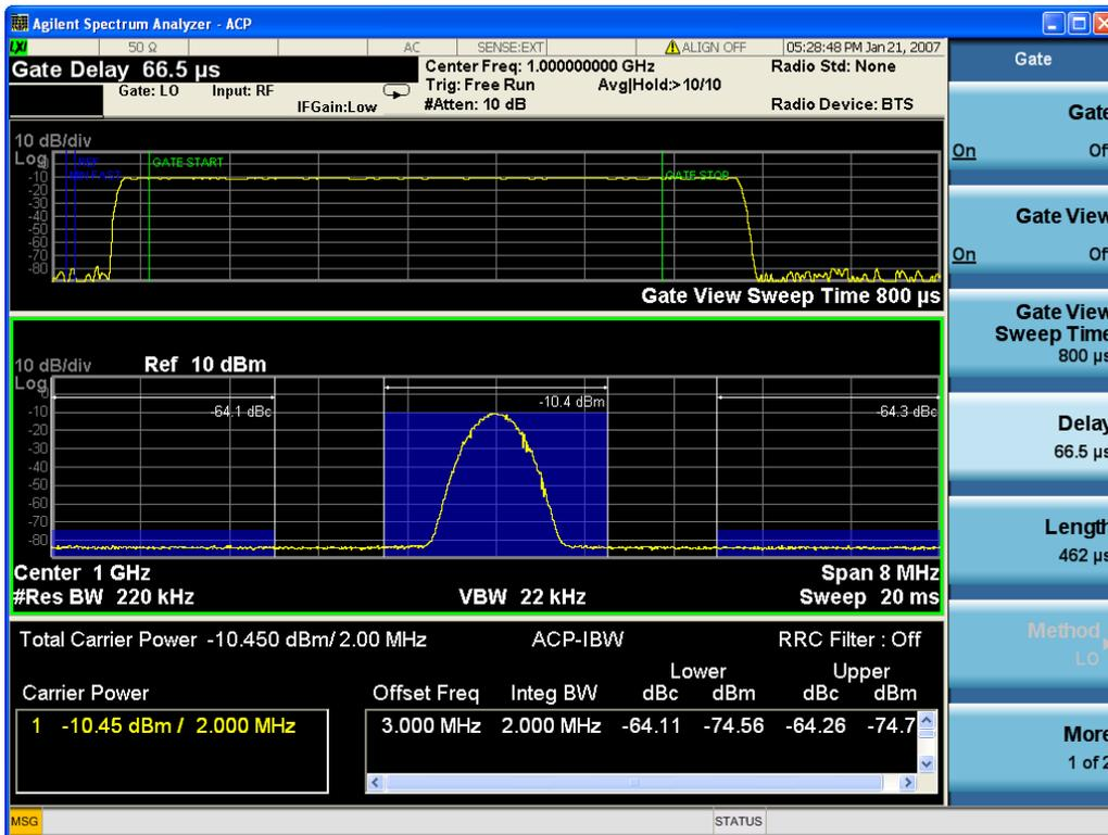
Turning Gate View off returns the analyzer to the Normal measurement view.
