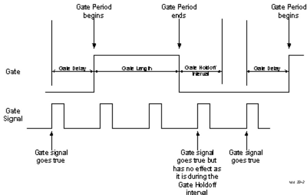
When Gate Holdoff is in Auto, the wait time calculated by the analyzer is used. When Gate Time is in Manual, the user may adjust the wait time, usually decreasing it in order to achieve greater speed, but at the risk of decreasing accuracy.
