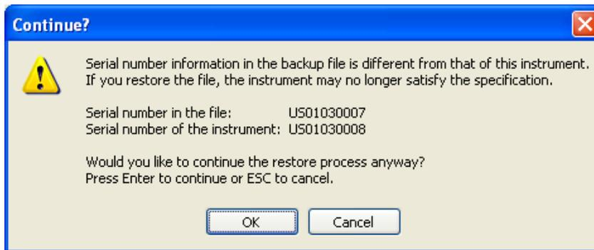
The default restore location will be first drive identified as an external drive (USB or LAN) if such is available; if not, the internal D: partition will be selected. The default restore file will be the most recent file that matches the default backup file name format: AlignDataBackup\_<model number>\_<serial number>\_<date>.bak
