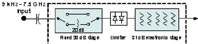
You can tell which attenuator configuration you have by pressing the Attenuation key, which (in most Modes) opens the Attenuation menu. If the first key in the Attenuation menu says Mech Atten you have the dual attenuator configuration. If the first key says Atten you have the single attenuator configuration.
