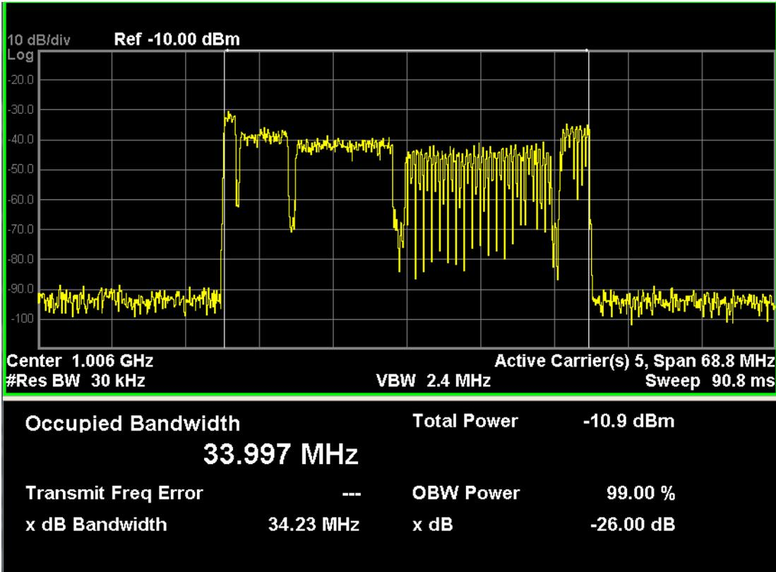
The number of active carriers is displayed to show how many carriers are identified as active in auto detected mode of span, otherwise “-” is displayed to indicate that it is out of scope.
