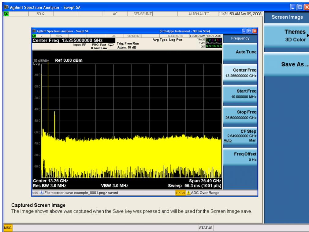
When you continue on into the Save As menu and complete the Screen Image save, the image depicted in the thumbnail is the one that gets saved, showing the menus that were on the screen before going into the Save menus. The save is performed immediately and does not wait until the measurement is complete.
