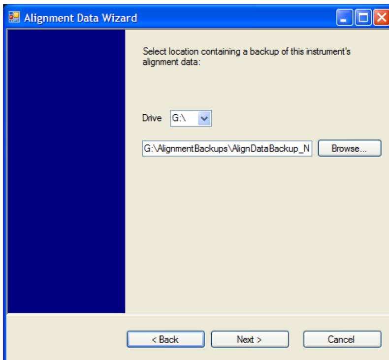
Changing the drive letter also modifies the path displayed in the box below. When this step is first loaded, the drive drop-down menu is populated with connected drives, which provide you with read access. The path defaults to the AlignBackups folder. The most recent \*.bak file in the folder will also be selected by default.
