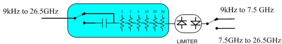
(note that Configuration 2 is not strictly speaking a dual-section attenuator, since there is no electronic section available. However, it behaves exactly like Configuration 1 without the Electronic Attenuator option EA3, therefore for the sake of this document it is grouped into the "Dual Attenuator" configuration)
