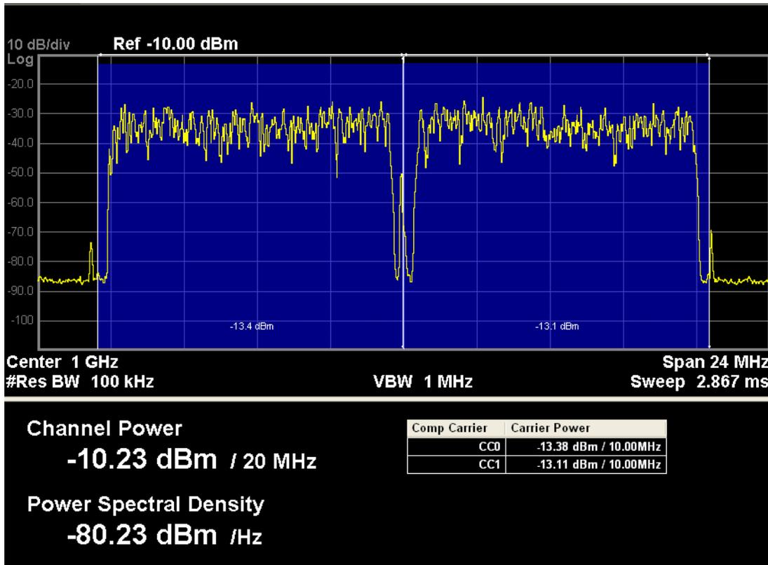
Figure 0-18 Power Results View of LTE-Advanced FDD/TDD CHP
