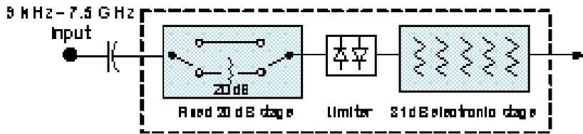
You can tell which attenuator configuration you have by pressing the Attenuation key, which (in most Modes) opens the Attenuation menu. If the first key in the Attenuation menu says Mech Atten you have the dual attenuator configuration. If the first key says Atten you have the single attenuator configuration.
