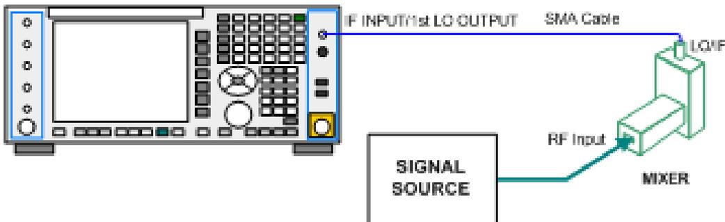
Legacy HP/Agilent and some third party mixers have separate LO In and IF out connections. This requires you to use an external diplexer to connect these mixers. A diplexer can easily be purchased for this purpose (for example, Diplexer Model # DPL.26 or # DPL.313B from OML Inc., Morgan Hill CA)
