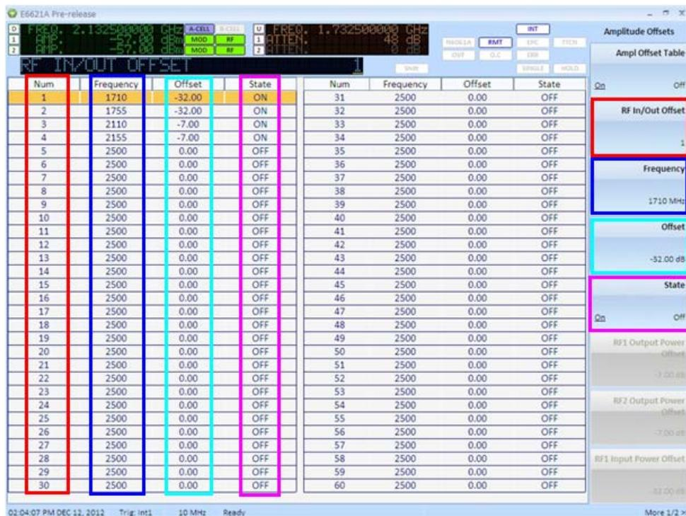
Figure 2 – 1: Offsets Applicable to Band 4 Frequencies
