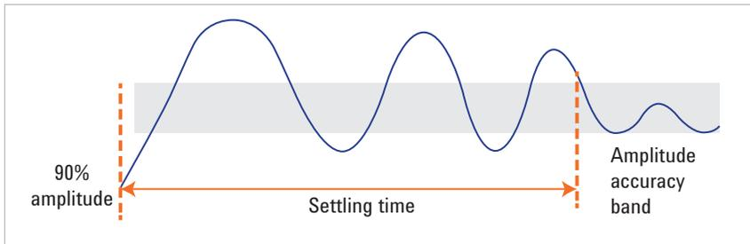
Figure 13. Settling time
