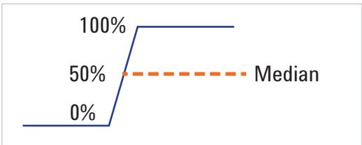
Figure 2. Time reference at median amplitude
