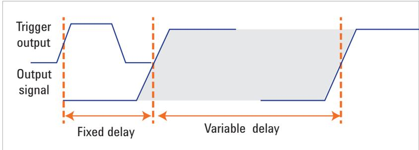
Figure 7. Pulse delay
