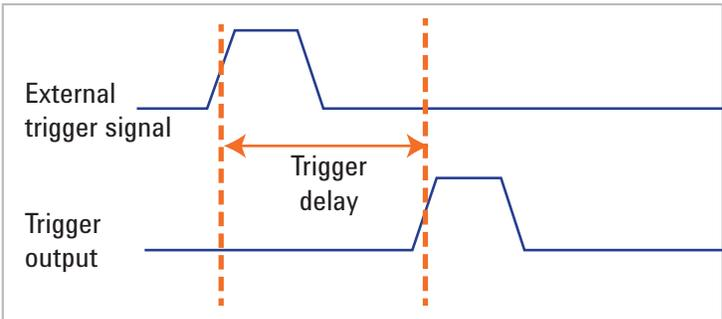
Figure 4. Trigger delay
