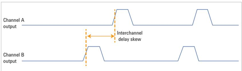
Figure 9. Interchannel delay
