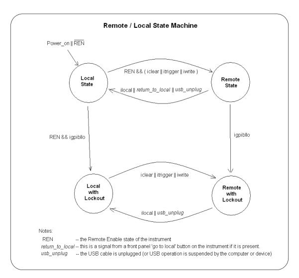
The following SICL functions are used to control the Remote/Local state transitions in USBTMC-USB488 devices sessions. (See the *SICL Online Help* for specific information on these functions.)
