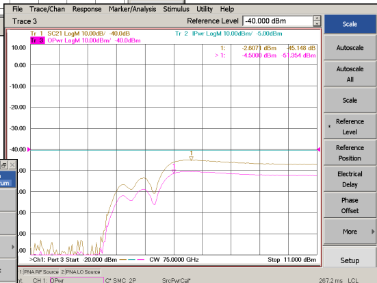
FIGURE 3a. This S21 plot results while sweeping the LO from -20 to +11 dBm at a mmWave frequency of 75 GHz.
