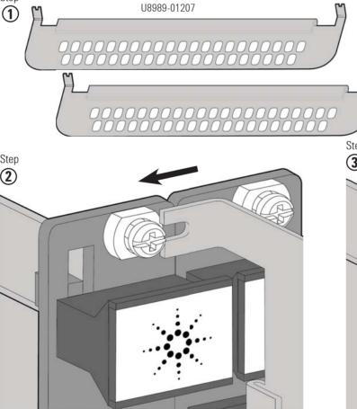
Insert the SLU card strain relief bracket's grooves behind the screws.
