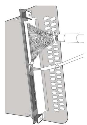
Using cable ties, tie the interface cables to the holes on the SLU card strain relief bracket
