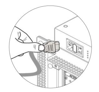
Plug the male end into a three-prong grounded electrical outlet. Ensure that the interface cables are connected and secure. Ensure that the power switch on the PXI subsystem is turned on as well on the DUT interface side.
