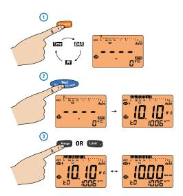
Polarization Index (PI) = IR  $_{10 \text{ minutes}}$  / IR  $_{1 \text{ minute}}$
