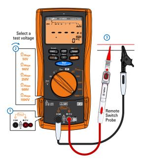
Insulation Resistance (IR) Test
