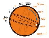
Turn the rotary switch from the or position to any other position to begin making measurements.
