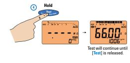
When an insulation test is in progress, the red LED indicator at the top of the tester will blink every 2 seconds (if the Limit function is not enabled).
