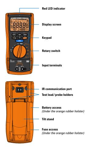
Using the Rotary Switch
