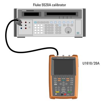
Set the calibrator output to 140 V. Wait a few seconds for the measurement to settle.
