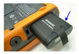
4 Install a new battery pack and re-assemble the battery access cover.
