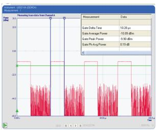
The time gated function enables measurement of peak, average, and peak-to-average ratio of a single burst signal for wireless signals such as Wimax, LTE, WLAN, MIMO.
