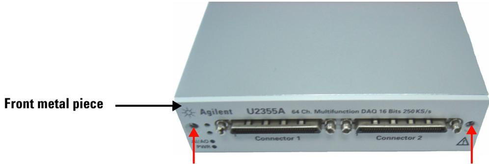
**Step 5: Gently pull the front metal piece out, which is attached to the carrier and measurement boards.**
