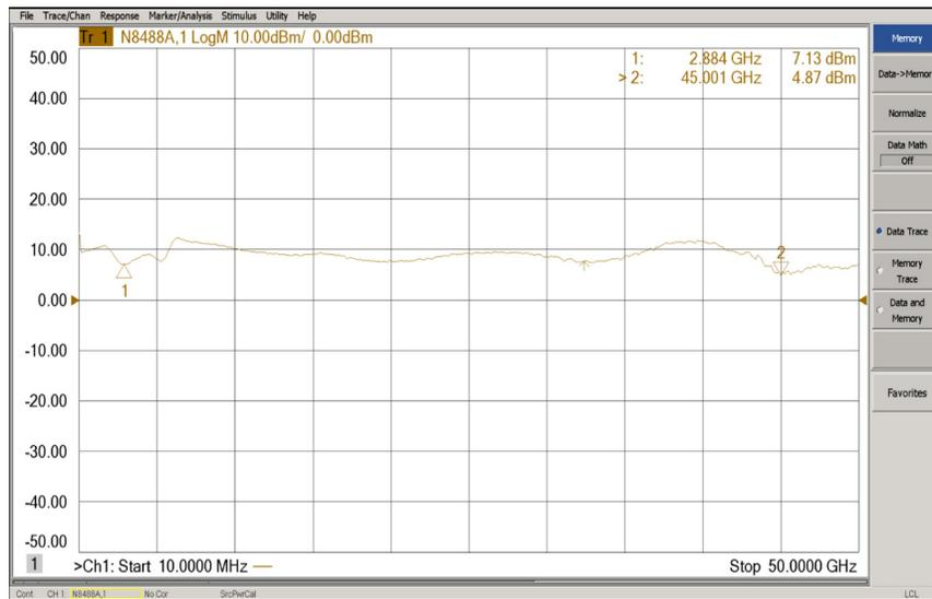
Figure 19 Typical Option 067 Port21 S-Parameter Plot
