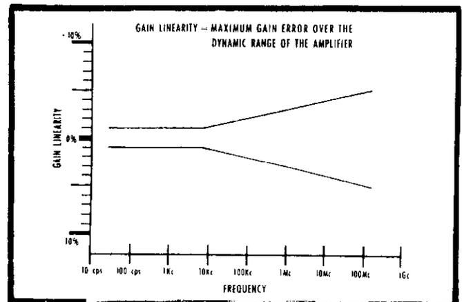
FIGURE 5. Models 108 and 109 Gain Linearity
