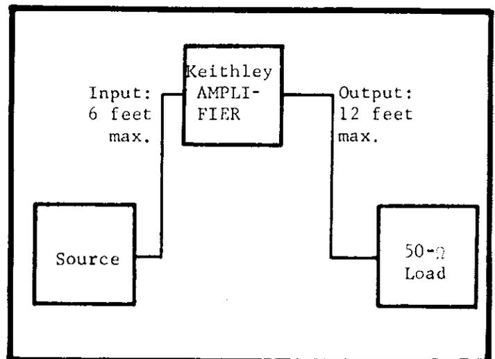
FIGURE 4. Amplifier Cable Connections. Maximum recommended cable length to input is six feet; from output, 12 feet. If longer cables are used, the specified flatness or overshoot may not be achieved. Use only coaxial cables.
