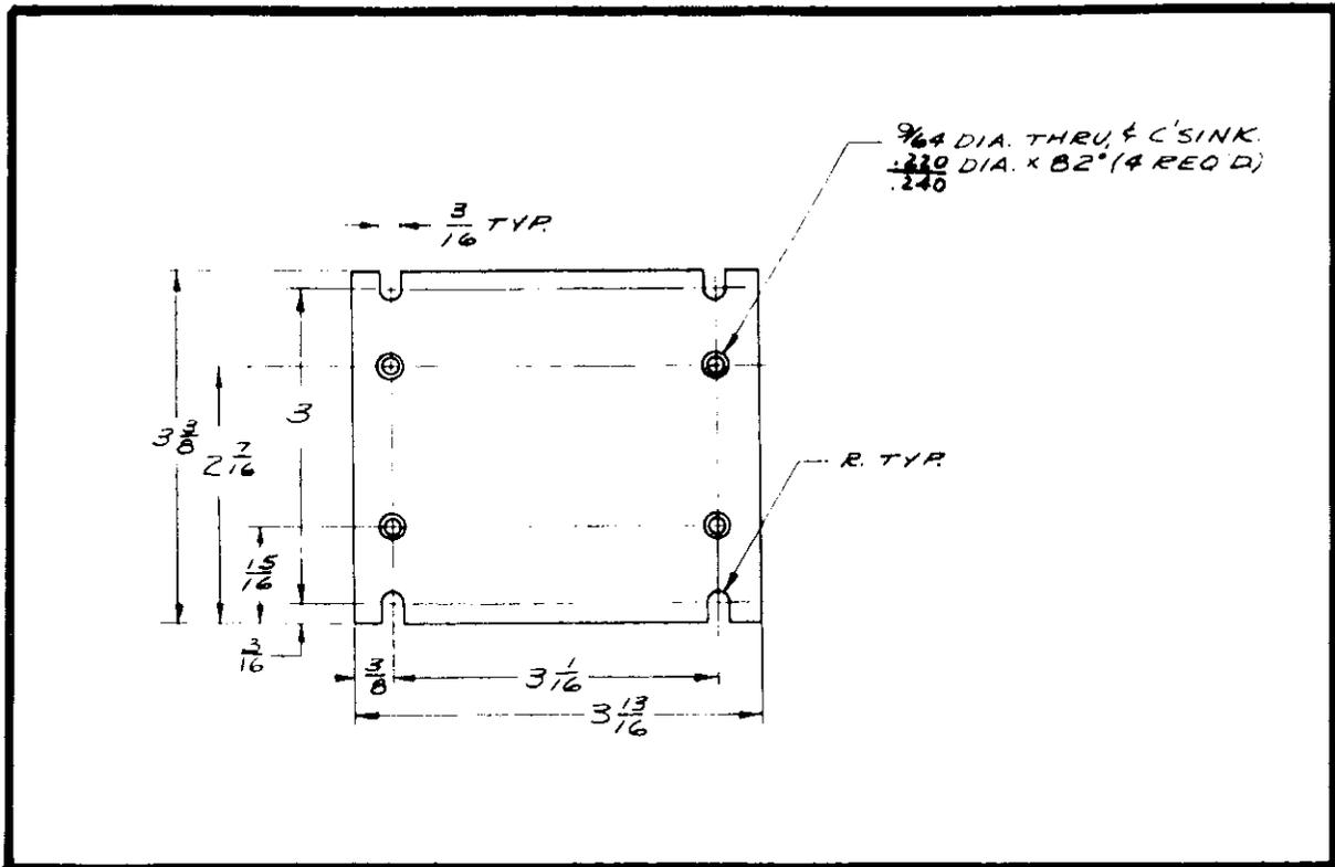
FIGURE 16. Dimensions of the Model 1082 Mounting Plate.
