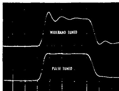
FIGURE 10. Models 108 and 109 Overshoot Characteristics. The Model 108 is wide-band tuned; the Model 109, pulse tuned. The oscilloscope is set for 5 nsec/cm horizontal, 0.2 v/cm vertical. The pulse amplifier has minimum pulse distortion at the expense of flatness (see Figure 9).
