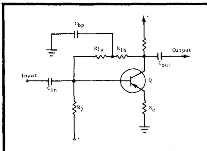
FIGURE 6. Basic Amplifier Stage. The diagram shows the stage design used in the 2-stage amplifier. Resistors  $R_1$  and  $R_2$  and the collector bias voltage drop provide a bias voltage divider, which stabilizes the base voltage. Resistor  $R_1$  supplies dc feedback. To eliminate degeneration caused by the ac feedback,  $R_1$  is divided into two parts,  $R_{1a}$  and  $R_{1b}$ . Capacitor  $C_{bp}$  bypasses the ac from the midpoint to ground.
