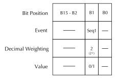
$\begin{array}{ll} \mbox{Value}: \ 1 = \mbox{Enable Negative Transition} \\ 0 = \mbox{Disable Negative Transition} \end{array}$
