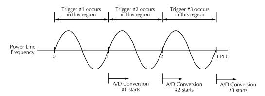
Note: A/D conversions assume an integration time of  $\leq$  1 PLC (Power Line Cycle)
