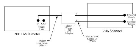
Figure 3-32 Connections using Trigger Link adapter
