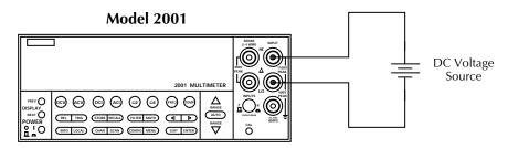
Input Resistance =  $10M\Omega$  on 1000V and 200V ranges; >  $10G\Omega$  on 20V, 2V and 200mV ranges.
