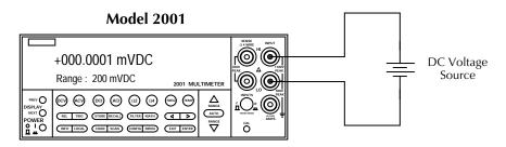
$\begin{array}{ll} \mbox{Input Resistance} &= 10 M\Omega \mbox{ on } 1000 \mbox{V} \mbox{ and } 200 \mbox{V} \mbox{ ranges} \ ; \\ &> 10 G\Omega \mbox{ on } 20 \mbox{V}, 2 \mbox{V} \mbox{ and } 200 \mbox{mV} \mbox{ ranges}. \\ &= 1 M\Omega \mbox{ on } DCV \mbox{ peak spikes measurement}. \end{array}$
