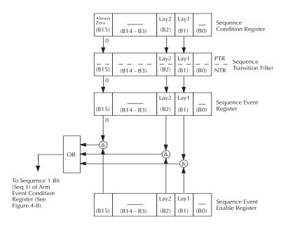
Lay1 = Layer 1 (Set bit indicates that 2001 is in arm layer 1). Lay2 = Layer 2 (Set bit indicates that 2001 is in arm layer 2).
