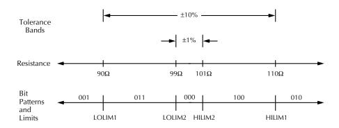
Figure 3-45 Using limit test to sort  $100\Omega$  resistors
