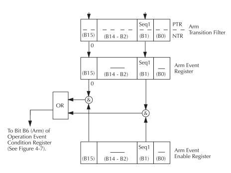
Seq 1 = Sequence 1 (Set bit indicates that the 2001 is in the arm layer of Sequence 1) & = Logical AND
