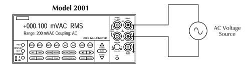
Input Impedance =  $1M\Omega$  shunted by <140pF
