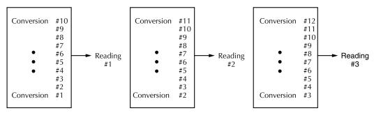
**B.** Moving filter mode; Type - Average, Readings = 10
