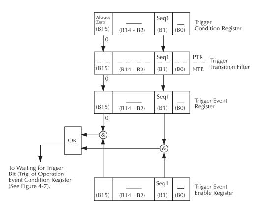
Seq 1 = Sequence 1 (Set bit indicates that the 2001 is in the trigger layer of Sequence 1)
