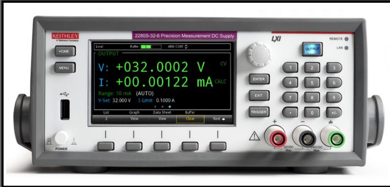
The Series 2280S Precision Measurement, Low Noise, Programmable DC Power Supplies are much more than just sources of clean power; they are also precision measurement instruments. They can source stable, low noise voltages as well as monitor load currents over a wide dynamic range from amps to nanoamps. The Model 2280S-32-6 can output up to 32V at up to 6A; the Model 2280S-60-3 can output up to 60V at up to 3.2A.
