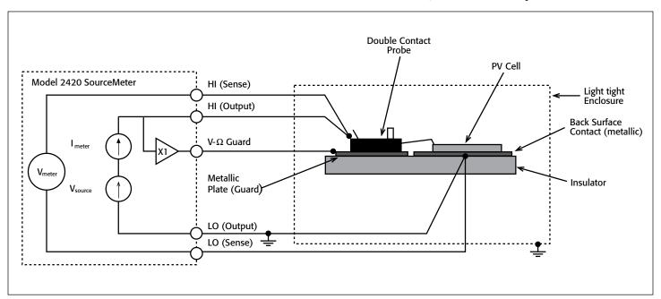
Figure 4: Guarded circuit configuration for dark reverse currents <1mA
