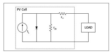
Figure 1: Equivalent circuit model of a photovoltaic cell
