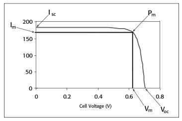
Figure 2: Forward bias I-V characteristics of a typical Si PV cell
