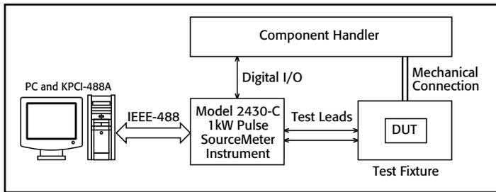
Figure 3. Model 2430-C based varistor production test system.
