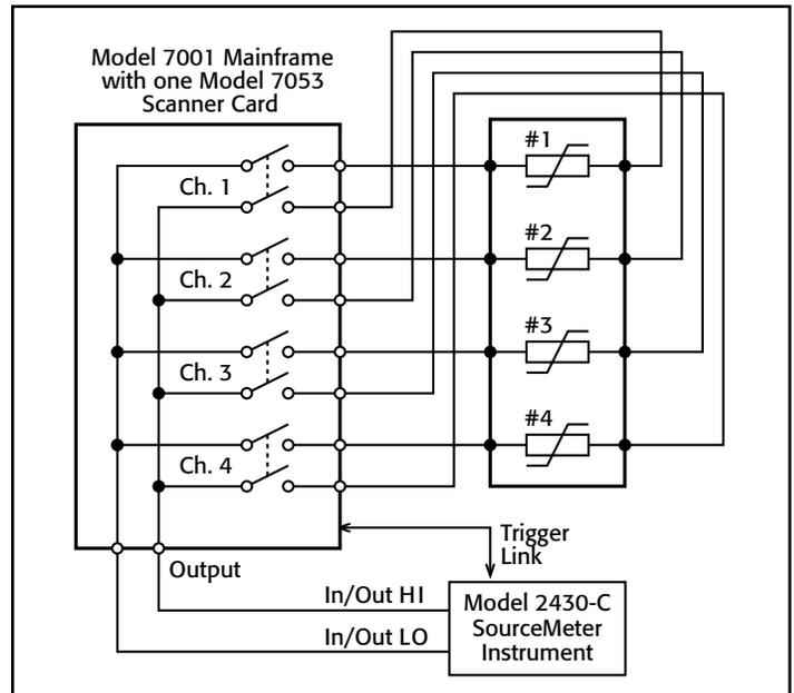
Figure 5. Using a switch mainframe for multi-point testing.
