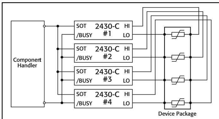
Figure 4. System diagram for testing a 4-device package.
