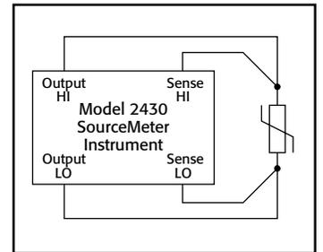
**Figure 9. Four-wire connection.**
