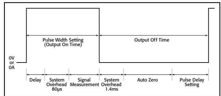
**Figure 7. Pulse width components for Model 2430-C output (Not to scale).**
