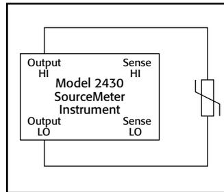
**Figure 8. Two-wire connection.**
