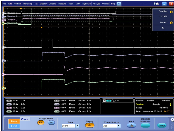
Figure 3: Close-up view of the start of the CI 230 waveforms from the Keithley Model 2612B System SourceMeter SMU instrument
