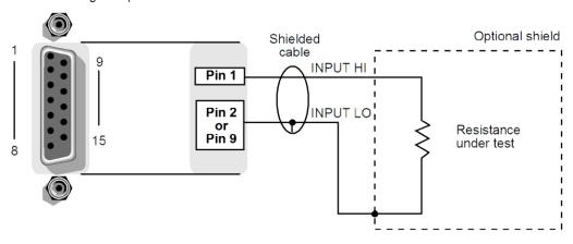
NOTE Source current flows from the connector HI to the connector LO pins.
