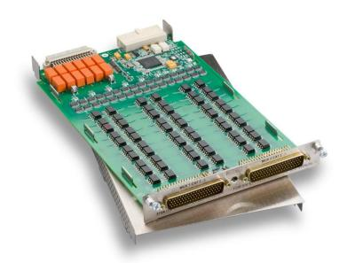
Figure 9-37: Model 3724 Dual 1x30 FET Multiplexer
