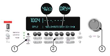
**NOTE** The Series 3700 is in 4-wire ohm mode when the  $4W\Omega$  is displayed. Dry Circuit is active when the DRY+ is displayed (see the above figure).
