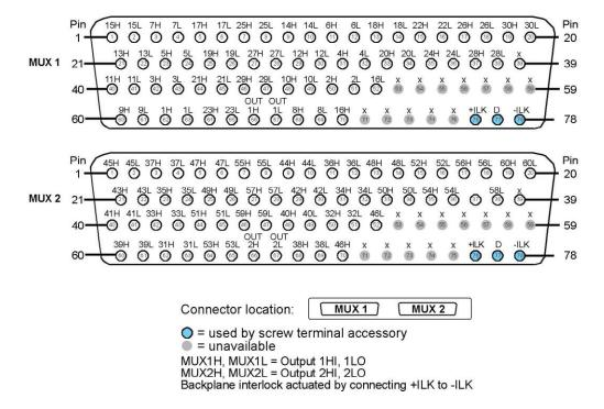
Figure 9-26: D-sub connection information for the Model 3723 (one-pole mode)
