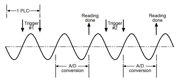
4-Wire Ohms are sensitive to 50 / 60 Hz power line noise, due to cabling and Model 3700 switch card loop area.
