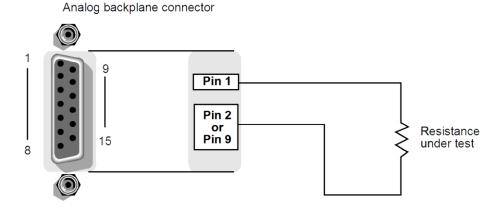
Connections to test continuity using a switching module are shown below. Because this is a 2-wire ohms measurement, Channels 1 through 40 of a 40-channel switching module can be used.
