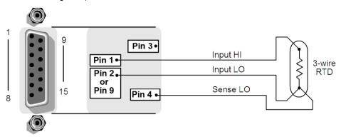
Figure 5-38: Three-wire RTD switching module connections
