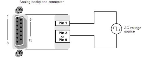
Figure 5-42: FREQ and PERIOD connections (switching module)
