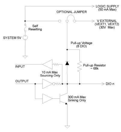
The figure shows a simplified schematic for one bit of a digital I/O channel. Each I/O bit has an optional pullup resistor in parallel with a diode that is used to clamp flyback voltages from inductive devices like electro-mechanical relays. However, when the optional jumper is removed, both the pullup resistor and diode are removed from the circuit. The pullup resistor is considered "weak" and can easily be overdriven by the external circuit.
