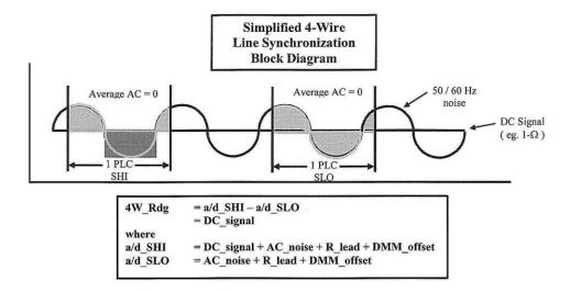
For Line Synchronization off and <1plc, reading rate increases, but measurement uncertainty and noise increases due to the Average AC noise during the SHI phase not cancelling with the SLO phase. With Line Synchronization ON, the SHI and SLO measurement phases are triggered at the rising edge of the power line zero crossing. This improves reading uncertainty and noise by >30x while minimal reading rate reduction.
