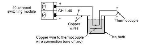
Figure 5-34: Internal reference junction (40 channel switching module)
