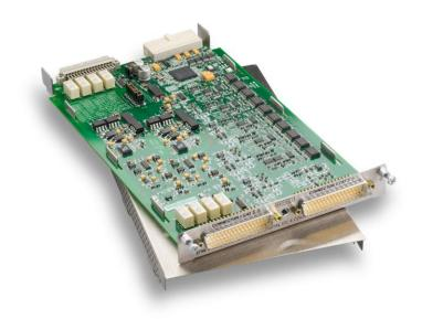
Figure 9-52: Model 3750 Multifunction I/O Card
