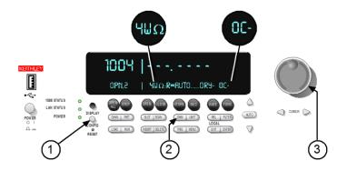
**NOTE** The Series 3700 is in 4-wire ohm mode when the  $4W\Omega$  is displayed. Offset compensation is active when the OC+ is displayed (OC- is shown in the above figure).
