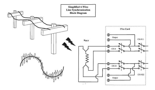
Traditional DMM 4-wire measurements are made in two phases, SHI and SLO. If the dmm.nplc=1 or a multiple of the power line, theoretically, the average AC noise is 0. Refer to the 4W-Rdg calculation (http://www.maximic.com/appnotes.cfm/appnote\_number/1041/).
