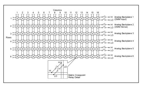
The channels on the 3730 are matrix channels. Unlike MUX channels, matrix channels do not have a DMM configuration associated with them. Therefore, specifying a matrix channel in the channel list parameter to the dmm.setconfig() function generates an error. To connect a DMM configuration to matrix channels, create a channel pattern with desired channels and analog backplane relays.
