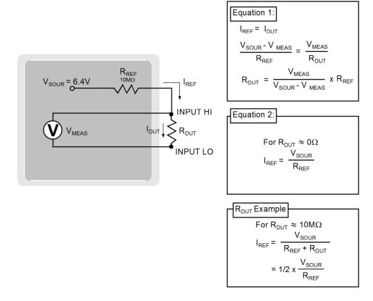
Because I = V/R, Equation 1 is modified using the V/R equivalents in place of  $I_{REF}$  and  $I_{DUT}$ . Therefore:
