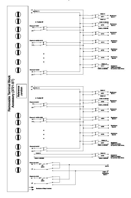
The following figure provides a switching schematic for the Model 3721 in 4-wire common side ohm mode.
