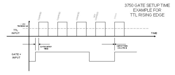
MINIMUM GATE INPUT SETUP TIME:
