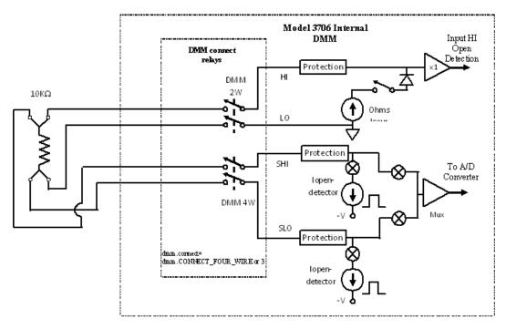
Figure 5-28: Model 3706 Internal DMM
