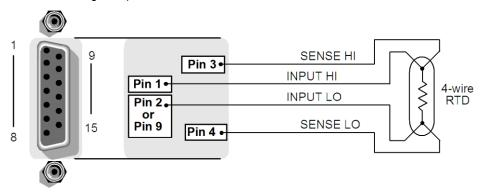
Figure 5-40: Four-wire RTD switching module connections
