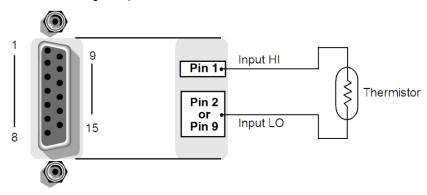
Figure 5-36: Thermistor switching module connection
