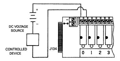
Figure 2. Typical PCM3 Connections (Channel 0 Shown)
