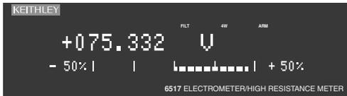
**Zero-centered Bar Graph** — The zero-centered bar graph is a graphical representation of the reading using plus/minus limits with zero in the center. Each full segment represents 10% of the limit.
