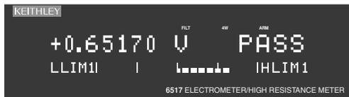
**Limits** — This display provides the result of the limit test. The graphical representation of the reading is shown on a zero-centered bar graph. If the reading is between the specified high and low limits, the PASS message is displayed. If the reading is outside of the limits, the FAIL message is displayed. Limits are set and enabled from the LIMITS option of the Main Menu.
