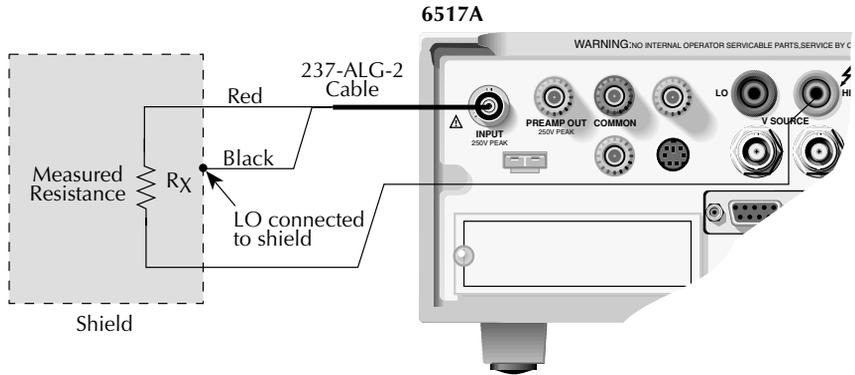
Note: V-Source low internally connected to electrometer low.
