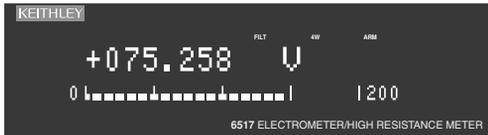
**Bar Graph** — The bar graph is a graphical representation of the reading with zero at the left end. Each full segment of the bar represents approximately 4% of the range limit.
