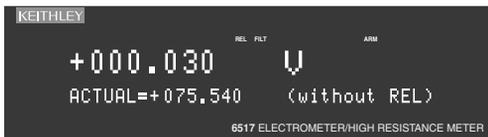
**Relative and Actual** — This display is used with the rel (relative) feature. While the top line shows the result of the rel operation, the bottom line shows the actual (raw) reading.
