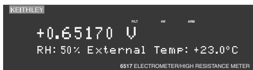
**Relative humidity and external temperature** — This display is used to display the relative humidity and external temperature readings. Note that the appropriate option has to be connected and enabled as explained in Section 1 of this manual.
