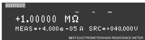
**Measure/source** — This display is used to display the measured current and the V-Source level for ohms measurements.
