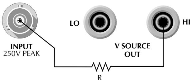
**Note:** V-SOURCE LO connected to ammeter input LO via METER-CONNECT option of CONFIGURE V-SOURCE Menu.
