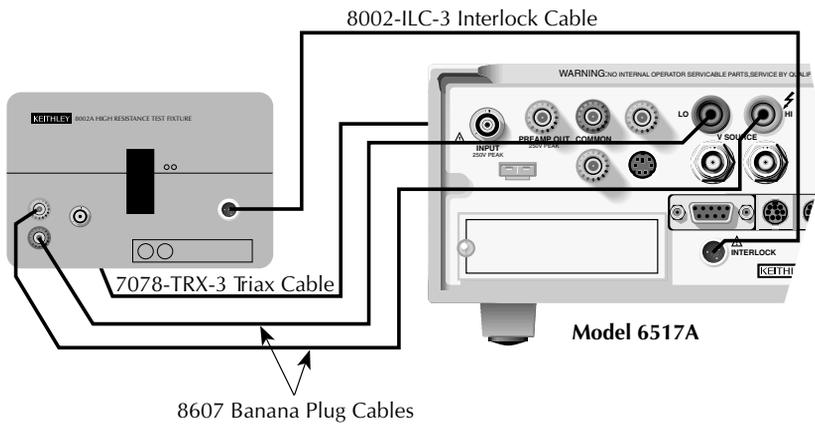
Warning: Connect ⊕ of fixture to safety earth ground using safety ground wire (supplied with 8002A test fixture).
