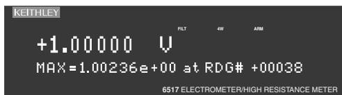
**Buffer** — When in RECALL, there are seven displays for buffer readings:
