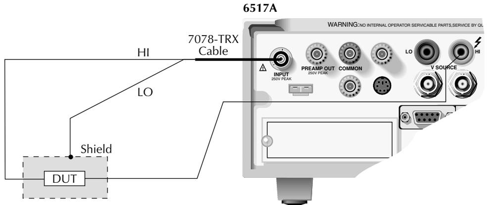
Note: Ammeter LO internally connected to V-source LO (see V-Source).
