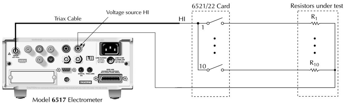
Note: Electrometer must be configured for internal voltage source connection
