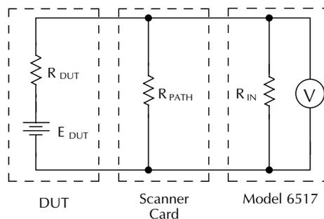
$R_{DUT}$  = Source Resistance of DUT
