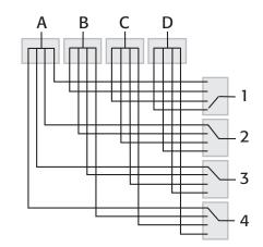
Figure 4. 4×4 Non-blocking switch
