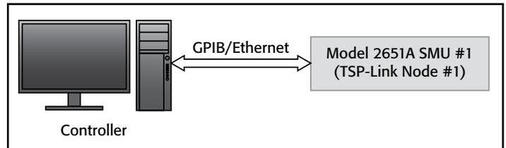
**Figure 5:** Communications setup for a single SourceMeter instrument.
