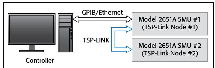
**Figure 6:** Communications setup for two Model 2651A instruments.
