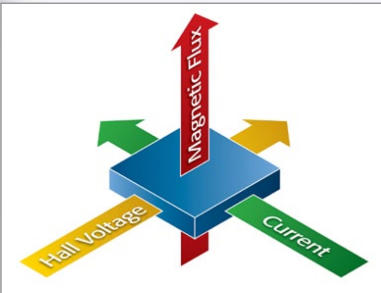
Figure 21: Illustration of Hall effect
