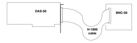
Figure 1. Cabling the DAS-50 to a BNC-50
