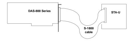
Figure 1. Connecting the DAS-800/CE Boards to an STA-U
