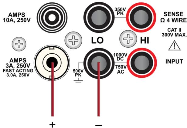
**Figure 99: Rear panel connections: Digitize current measurement (current below 10 A)**
