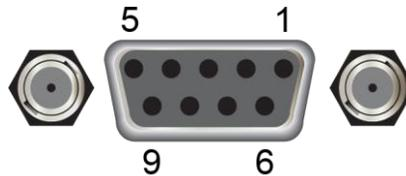
**DMM6500 digital I/O port pinouts**
