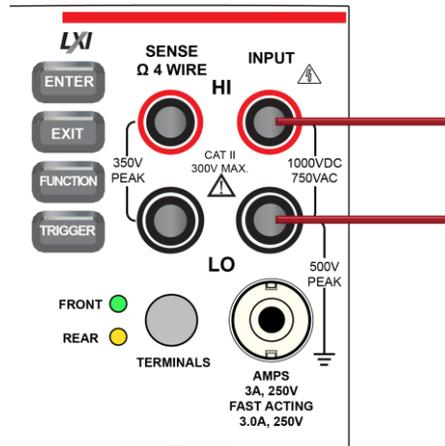
Figure 62: Rear panel connections: AC voltage measurement
