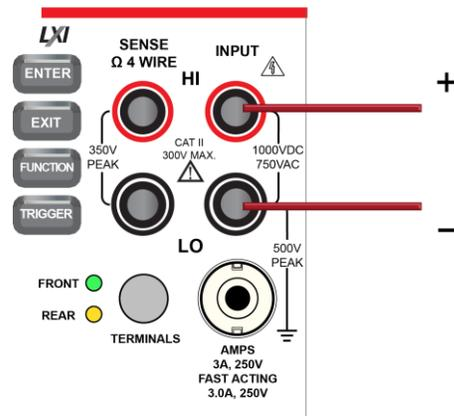
Figure 96: Rear-panel connections: Digitize voltage measurement
