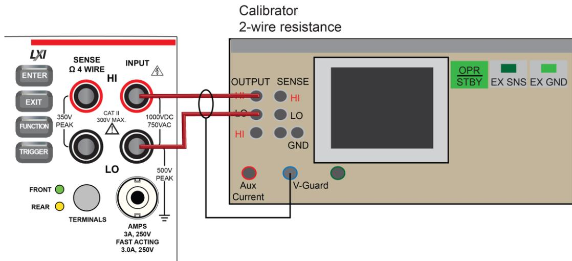
2. Set the calibrator for 2-wire resistance with external sense off.
