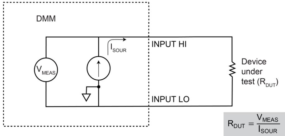
**Figure 106: Four-wire constant-current source method**
