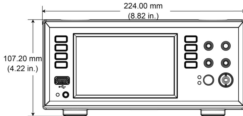
**Figure 3: DMM6500 dimensions side with bumpers installed**
