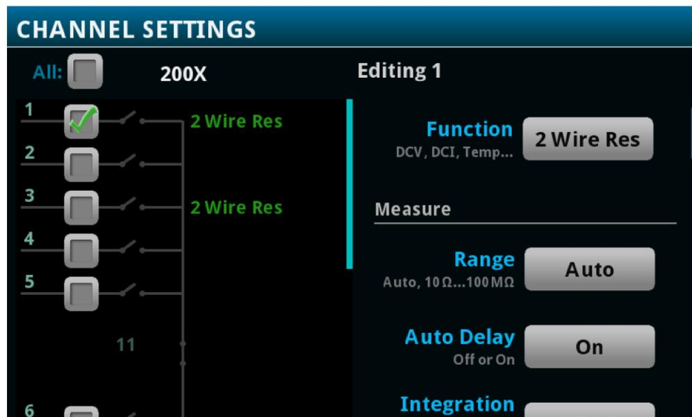
The Scan screen is ideal for configuring a whole scan. It includes options for the channels and the scan. You can also set up triggering to establish the flow of the scan using both the DMM6500 and external equipment. You can access the Scan screen by pressing MENU. Under Channel, select Scan. The figure below shows the Scan screen.
