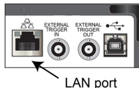
You can connect the instrument to the LAN in a one-to-one, one-to-many, two network cards, or enterprise configuration, as described in the following topics.
