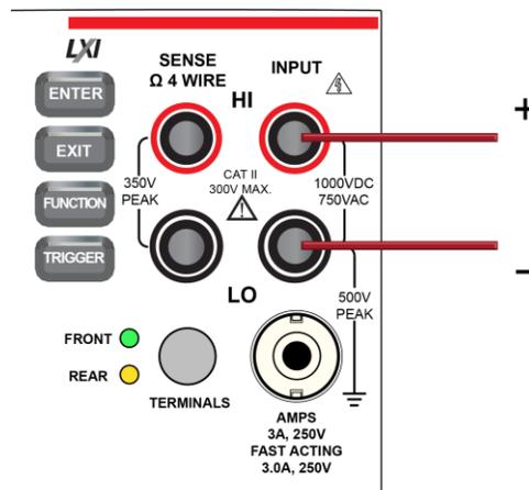
Figure 90: Rear panel connections: Capacitor measurement
