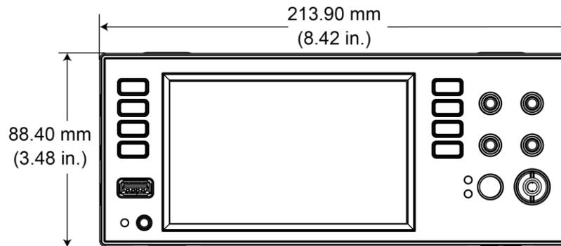
**Figure 5: DMM6500 side dimensions with bumpers removed**
