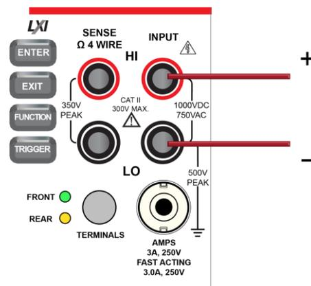
Figure 60: Rear panel connections: DC voltage measurement
