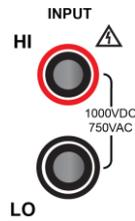
Use the INPUT HI and INPUT LO terminals for all measurements except current.
