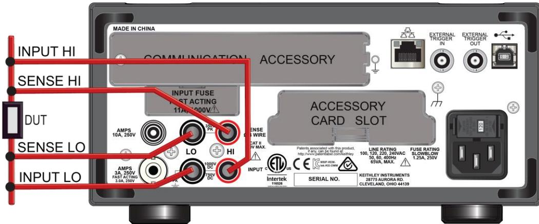
**Figure 74: DMM6500 front-panel 4-wire remote sense connections**
