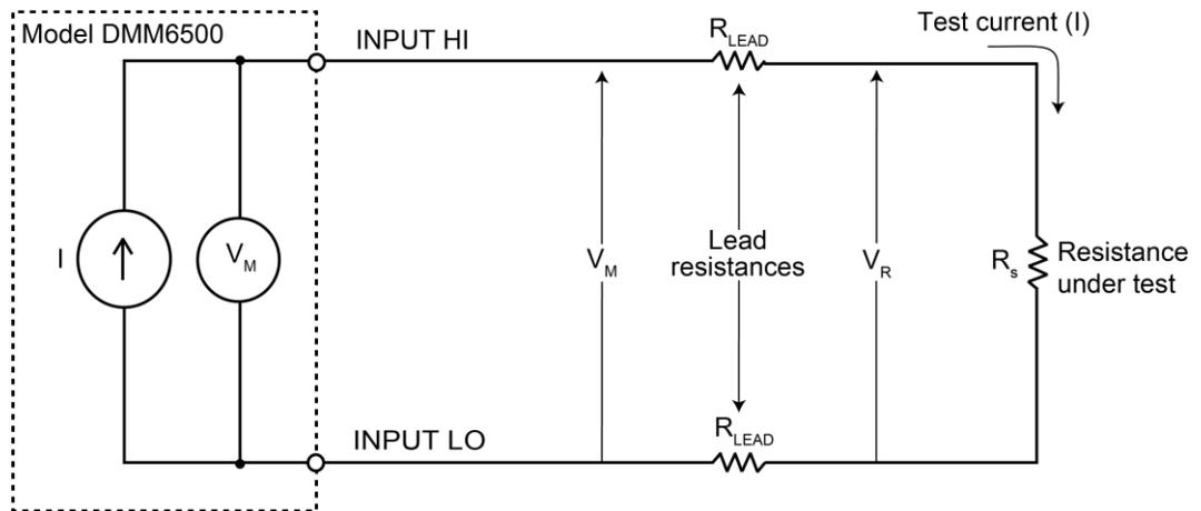
$$\text{Measured resistance} = \frac{V_M}{I} = R_s + (2 \times R_{LEAD})$$
