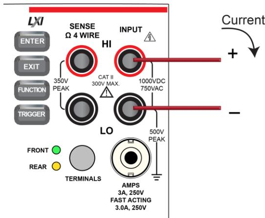
**Figure 80: Rear panel connections: Continuity measurement**
