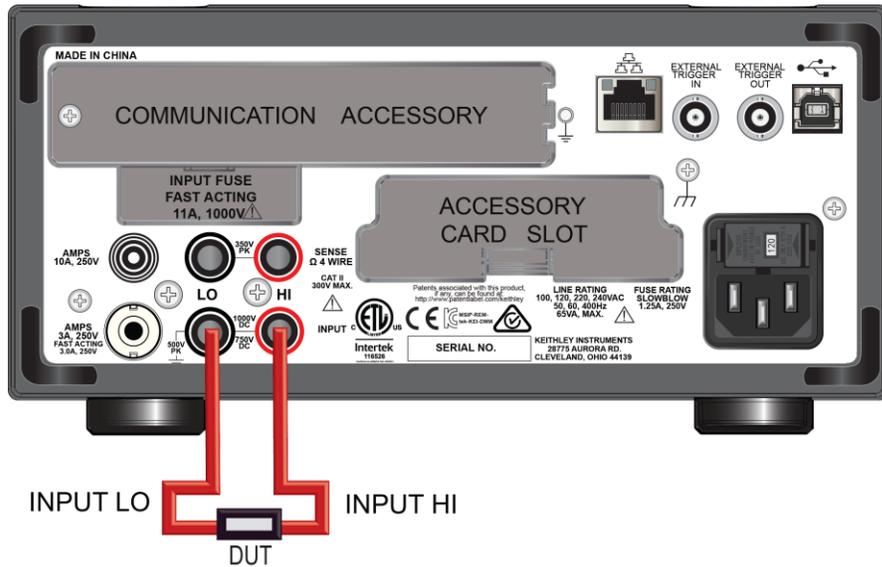
Figure 72: Two-wire DUT connections to the front panel
