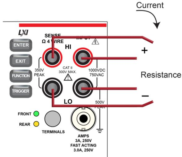
Figure 78: Rear panel connections: 4-wire resistance measurement
