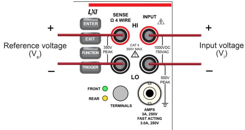
Figure 94: Rear panel connections: DC voltage ratio measurement
