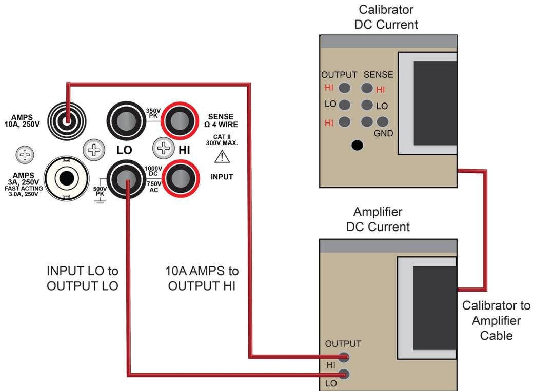
9. Enable the calibrator amplifier and select the **BOOST** key.
