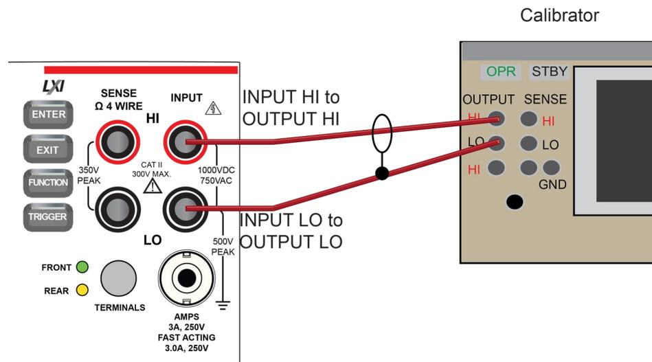
2. On the DMM6500, press the **FUNCTION** key and select **DC voltage**.
