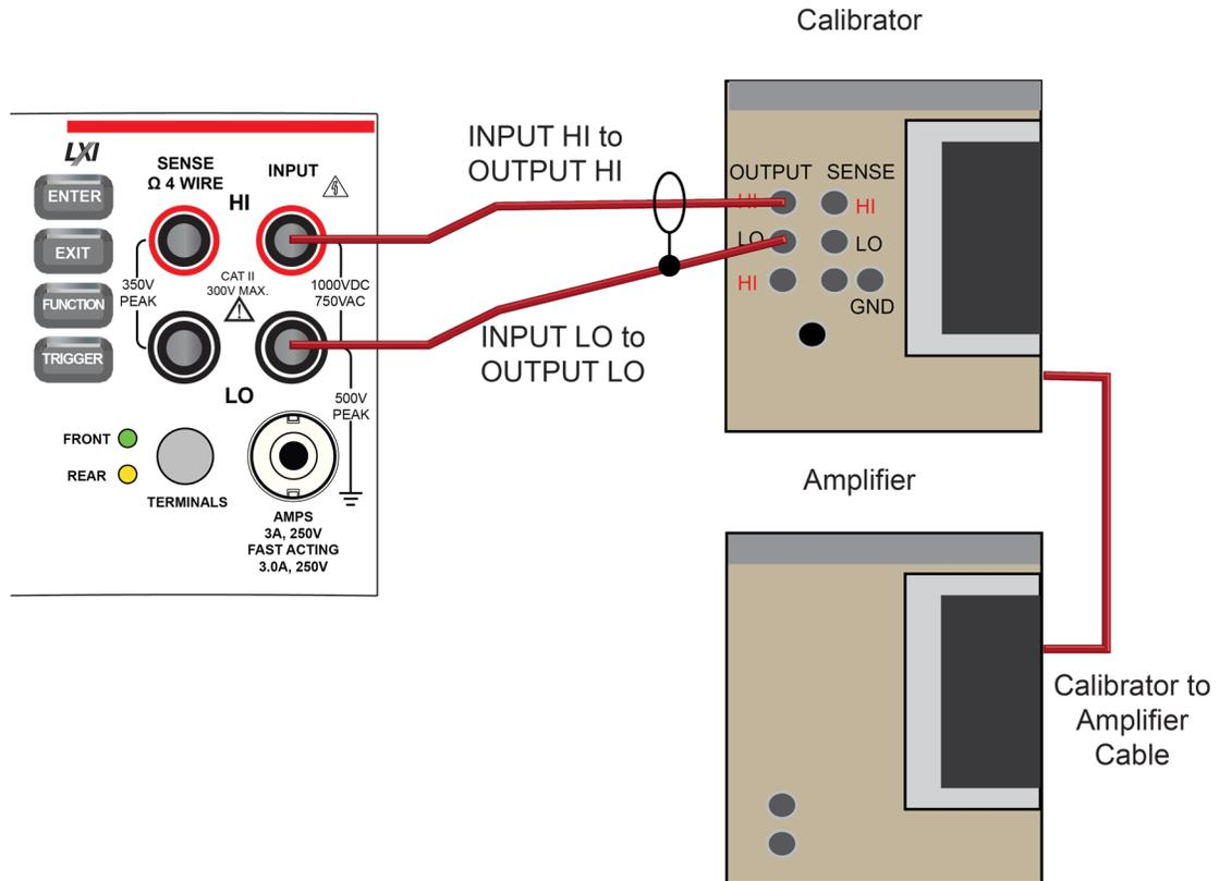
4. On the DMM6500, press the **FUNCTION** key and select **AC voltage**.
