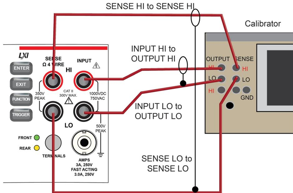
3. Allow the instruments and cables to settle for five minutes.
