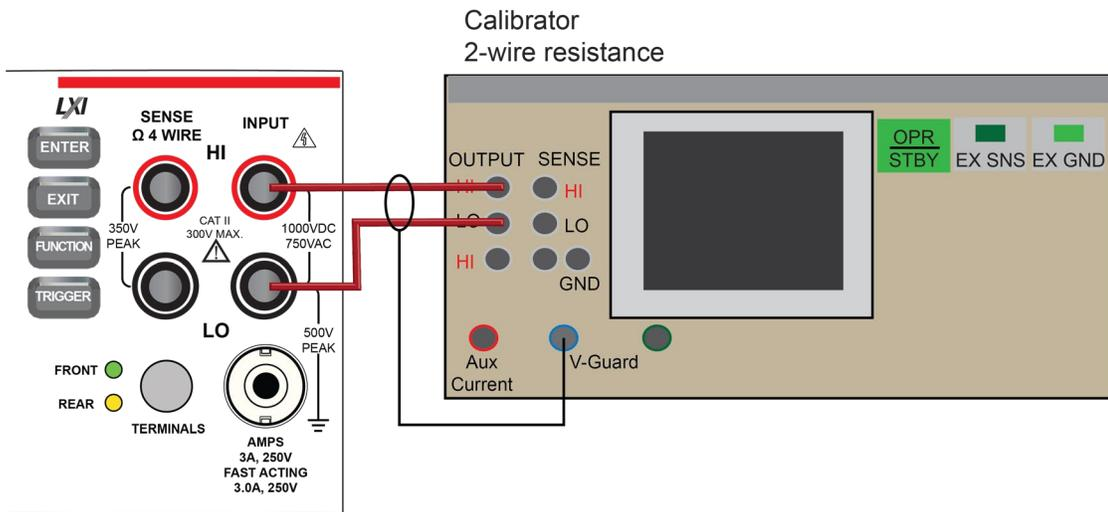
2. Set the calibrator for 2-wire resistance with external sense off.
