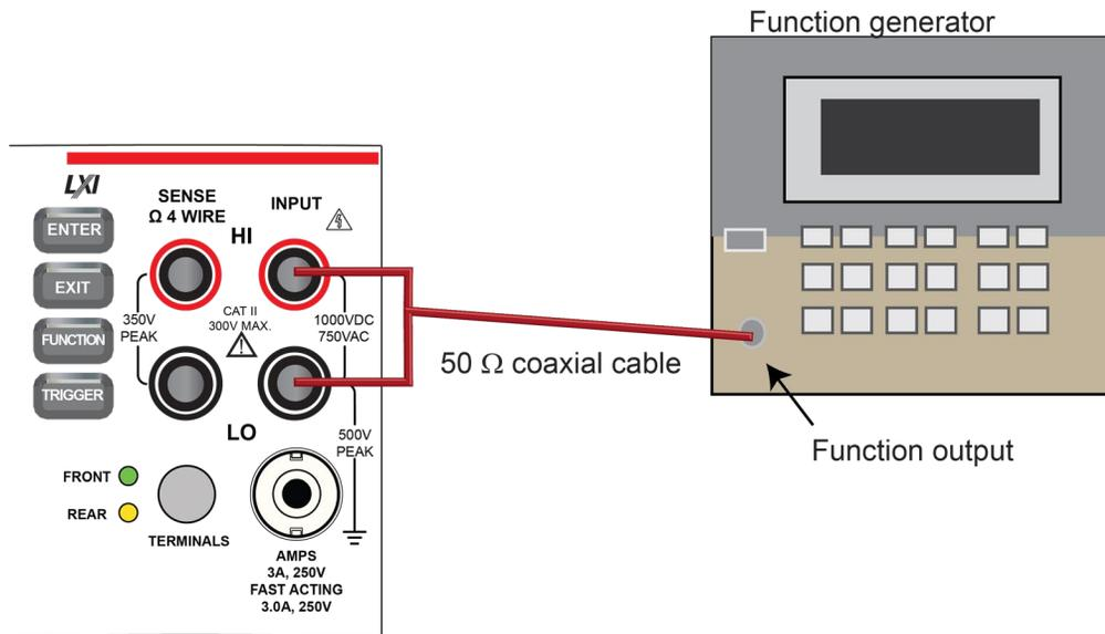
3. Set the function generator output impedance to high, amplitude of 5 V<sub>RMS</sub>, waveform to square wave.
