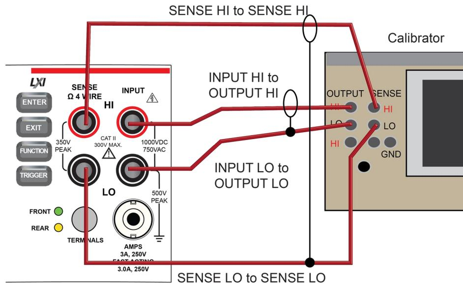
2. Set the calibrator for 4-wire resistance with external sense on.
