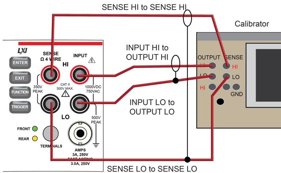
2. For 3-wire accuracy, connect the DMM6500 INPUT and SENSE terminals to the calibrator as shown in the following figure.
