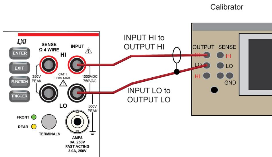
2. On the DMM6500, press the **FUNCTION** key and select **AC voltage**.
