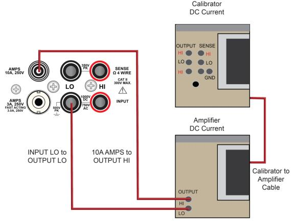
Figure 198: Connections for the 10 A range
