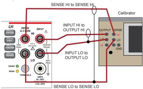
Figure 187: Connections for 4-wire resistance accuracy verification
