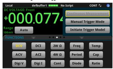
Figure 35: Trigger mode indicator
