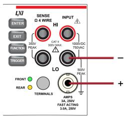
Figure 63: Front panel connections: DC current measurement (3 A or less)
