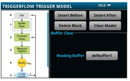
To see the parameters that you can change from the front panel, select a block in the trigger model diagram. The available options change depending on the type of block you select.
