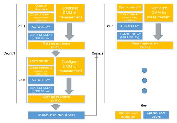
Figure 102: Example: Two-channel scan list with a scan count greater than 1
