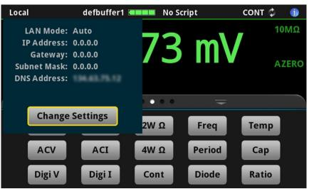
Figure 31: Communications indicator expanded
