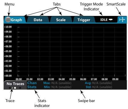
The swipe bar at the bottom of the Graph tab shows which buffers are providing the displayed data, the scale that is used, buffer statistics, and cursors.
