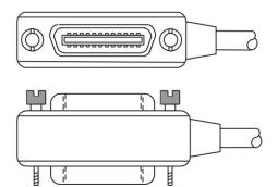
To allow many parallel connections to one instrument, stack the connectors. Each connector has two screws on it to ensure that connections remain secure. The figure below shows a typical connection diagram for a test system with multiple instruments.
