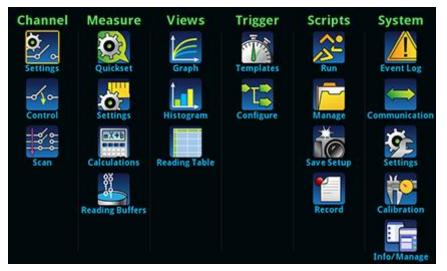
Figure 49: DMM6500 main menu - front terminals selected
