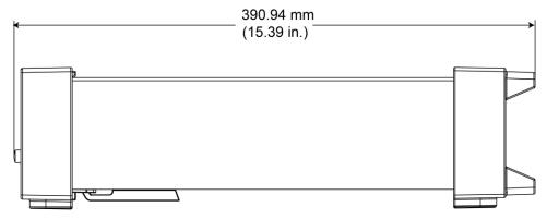
The following figures show the dimensions when the handle and bumpers have been removed.
