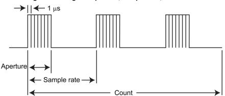
Figure 100: Digitize aperture, sample rate, and count
