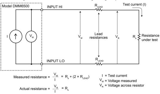
Figure 69: Two-wire resistance sensing for high impedance DUT
