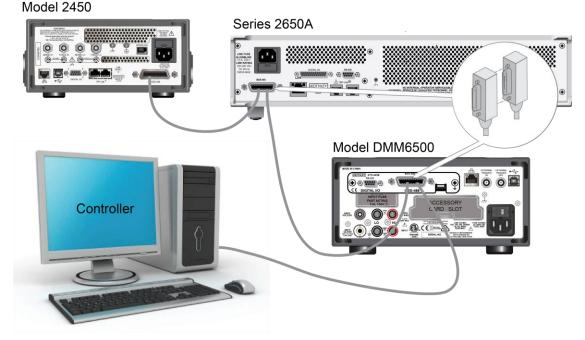
Figure 8: DMM6500 Instrument GPIB connections
