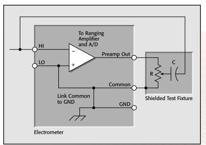
Figure 12: External Damping Circuit
