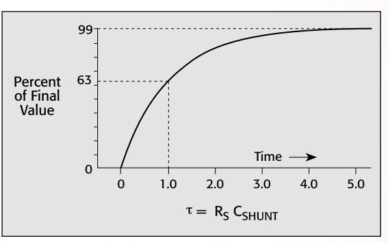
Figure 19: Exponential Settling Time Caused by Time Constant of Shunt Capacitance and Source Resistance
