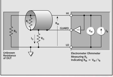
Figure 17: Guarding Cable Shield to Eliminate Leakage Resistance
