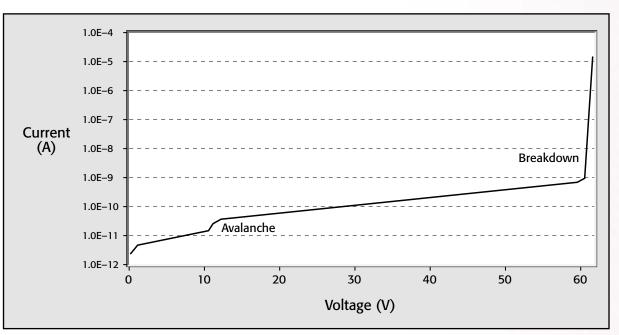
Figure 21: Current vs. Reverse Voltage Sweep of an InGaAs APD
