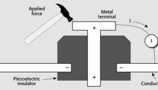
Figure 10: Piezoelectric Effect
