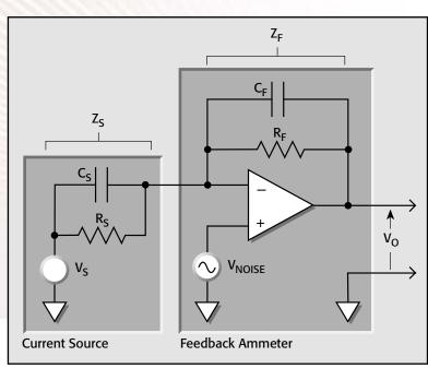
Figure 4: Simplified Model of a Feedback Ammeter
