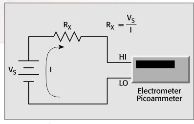
Figure 1: High Resistance Measurement Using External Voltage Source
