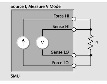
*Figure 15: Using the SMU in the Four-Wire Mode to* Measure High Resistance
