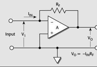
Figure 3: Feedback Ammeter
