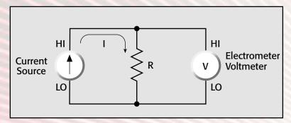
Figure 14: Constant-Current Method Using a Separate **Current Source and Electrometer Voltmeter**
