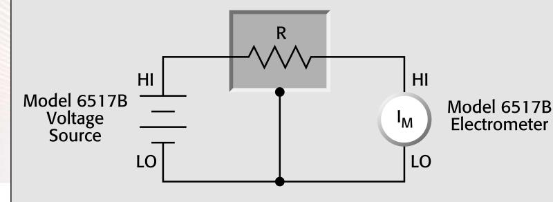
Figure 22: Connecting the Model 6517B Electrometer for Voltage Coefficient Testing
