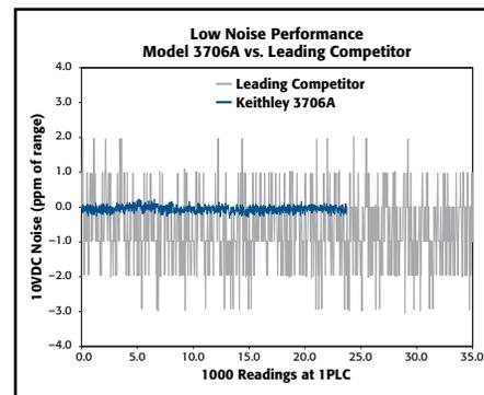
Compare the Model 3706A's 10V DC noise and speed performance with that of the leading competitor. All the data was taken at 1PLC with a low thermal short applied to the input, which resulted in 10× lower noise and 7× faster measurements for the Model 3706A.
