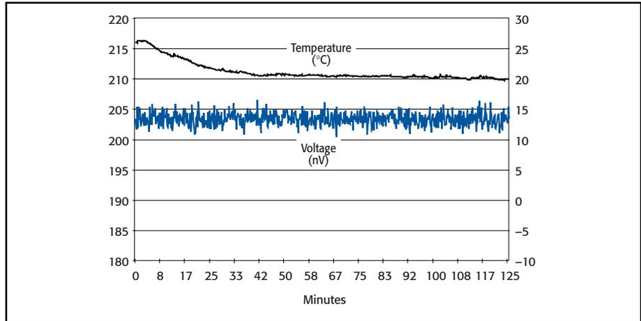
**Figure 5. The Model 2182A's delta mode provides extremely stable results, even in the presence of large ambient temperature changes. In this challenging example, the 200nV signal results from a 20µA current sourced by a Model 6221 through a 10mΩ test resistor.**
