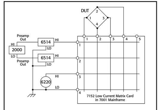
One Model 7152 Matrix Card, housed in a Model 7001 mainframe, is used to connect the electrometers and the current source to the sample. Two Model 6514 electrometers are used as unity gain buffers, and their output difference is measured with a Model 2000 DMM. To ensure faster measurement time, guarded measurements are made by turning the Guard switch ON for both of the Model 6514s, and by guarding the Model 6220 output. Call Keithley's Applications Department for cabling information.
