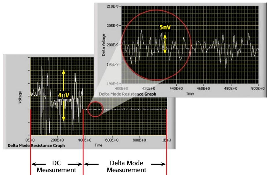
**Figure 2. Results from a Model 2182A/6220 using the delta mode to measure a 10mΩ resistor with a 20µA test current. The free Model 6220/6221 instrument control example start-up software used here can be downloaded from [www.keithley.com](http://www.keithley.com).**
