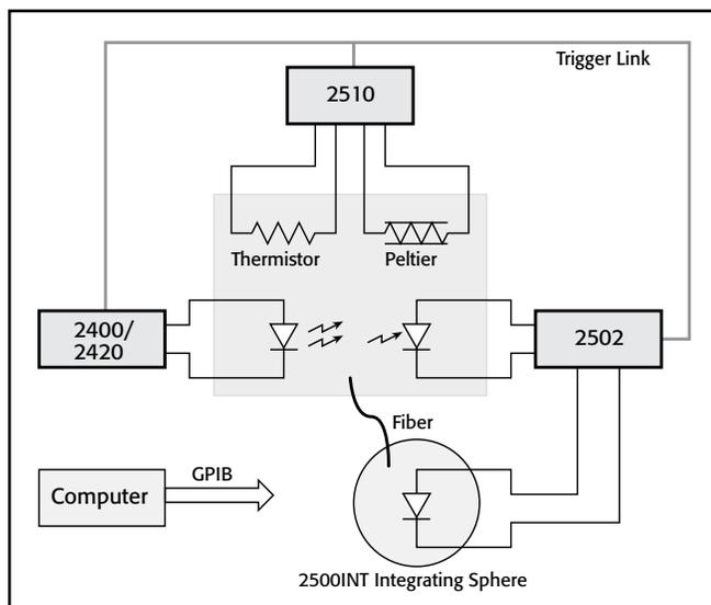
The Model 2502 is designed for tight integration with other Keithley instruments that are often used in LIV test systems for laser diode modules. These other instruments include the Model 2400 SourceMeter® and Model 2510 TEC SourceMeter SMU instruments.
