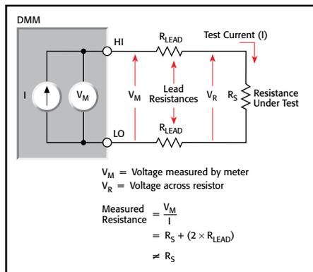
Figure 4a. Two-wire resistance measurement: Lead resistance error
