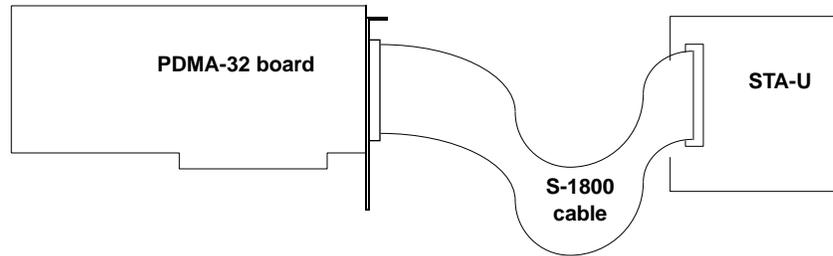
**Figure 1. Connecting a PDMA-32 Board to an STA-U**
