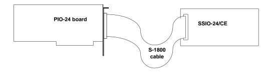
Figure 1. Connecting an SSIO-24/CE Accessory to a PIO-24 Board
