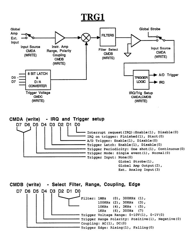
CMDC (write) - Trigger Voltage (0 - 255)
