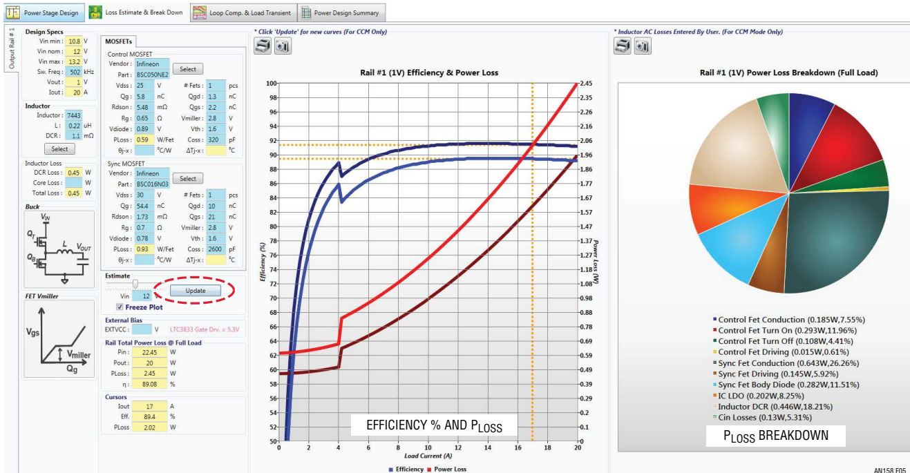
Figure 5. Design Step 3 – Optimize Efficiency and Power Losses
