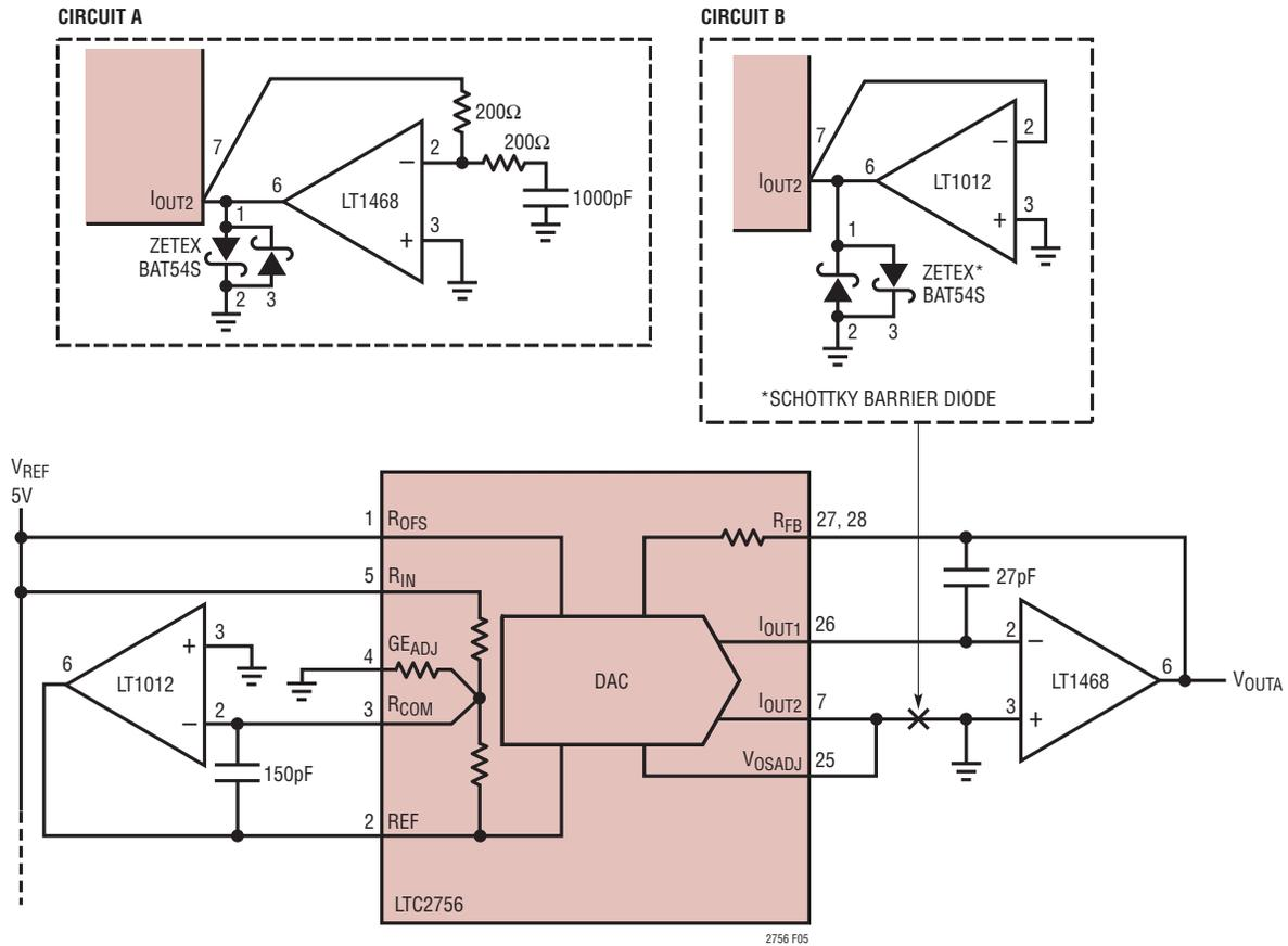
Figure 4. If a Low-Impedance GND Plane Is Unavailable, Drive I<sub>OUT2</sub> with a Force/Sense Amplifier As Shown. Use Circuit A to Minimize Impact on Settling Time, or Circuit B for Lower Power Consumption and Better Accuracy
