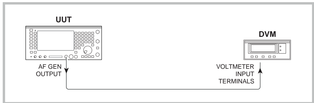
Fig. 5-10 Audio generator level accuracy checks
