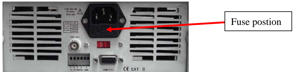
Picture 3.1 Fuse Location
