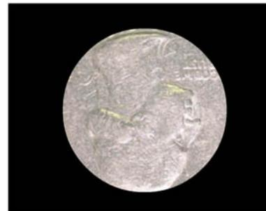
Sometimes vignetting cannot be eliminated completely because the difference in size between the camera aperture and the phototube is just too large to accommodate or other factors.
