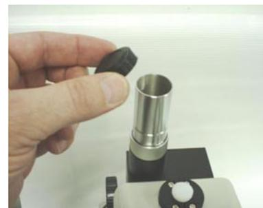
Now we will **place the camera** setup onto the trinocular tube.
