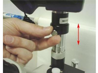
Once the camera is parfocal to the microscope, it should not have to be re-adjusted.
