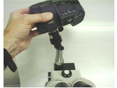
Your camera will need to be parfocalled with the microscope which is accomplished by **adjusting the height** of the camera on the tube. To do that, we are going to first check or parfocal the microscope by placing a specimen on the stage.
