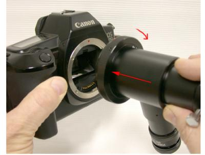
The next step is to install the photo eyepiece onto the trinocular tube.
