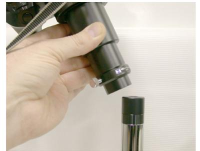
With the adapter in place, use the locking set screw to secure the installation.
