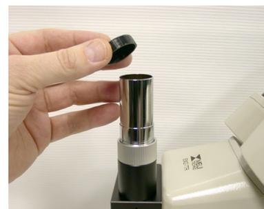
Next, we **screw on the camera adapter ring** onto the camera attachment.
