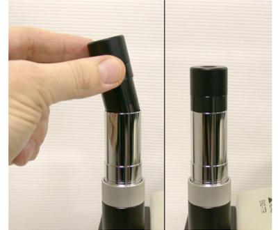
Take your camera with the adapter tube installed and slide it on top of the tube with the photo eyepiece in place.
