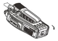
To remove the battery pack, press the battery latch backwards, and then remove the battery away from the radio.
