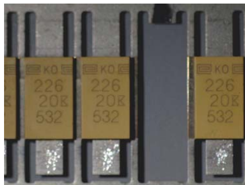
Figure 13. Epoxy Case Molded around Assembled Capacitor and Laser Printed.
