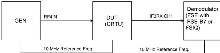
Fig. 1-6 Test setups for RX demodulation measurements
