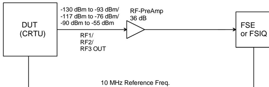
Fig. 1-2 Test setups for TX level measurements
