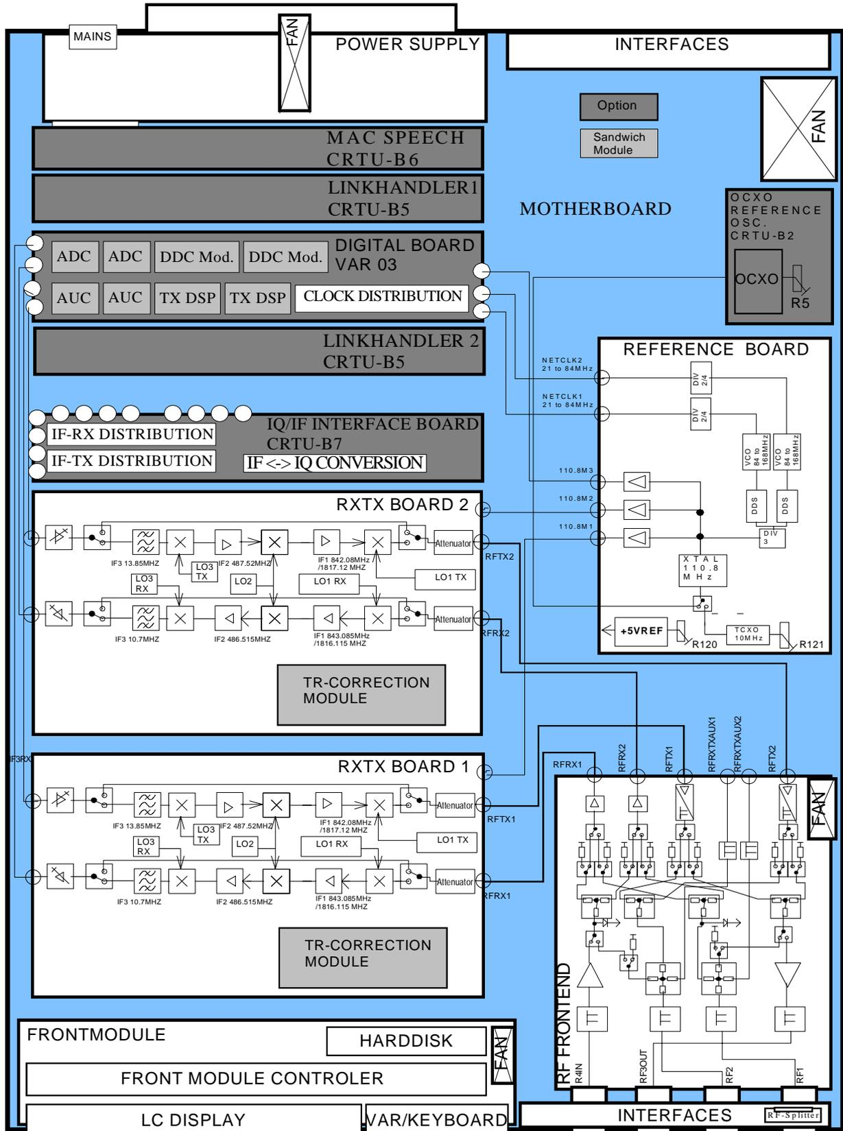
Fig. 3-1 Block diagram of CRTU Radio Unit
