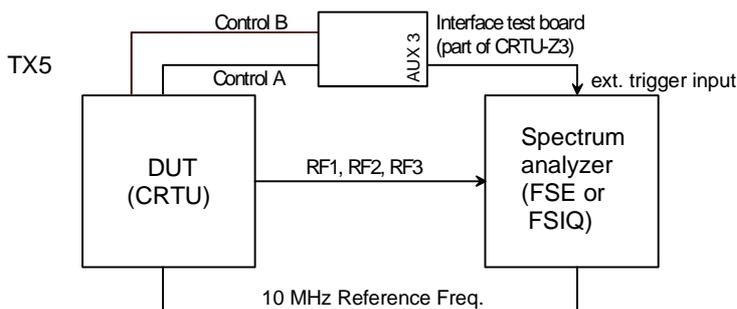
Fig. 1-3 Test setups for general TX measurements
