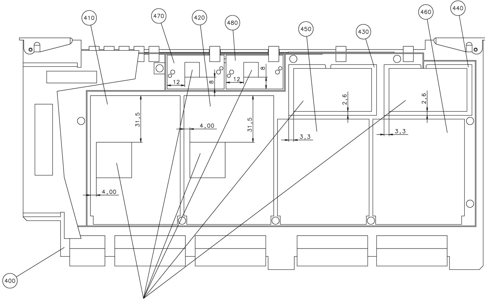
Affix the supplied heat conducting mat with its adhesive side to the sandwich module as shown
