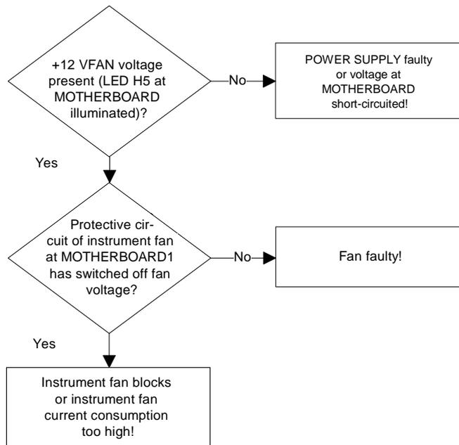
**Note:** *Measure instrument fan voltage at connector X 211! By pressing the STANDBY/ON key again, the protective circuit of the instrument fan can be restarted.*
