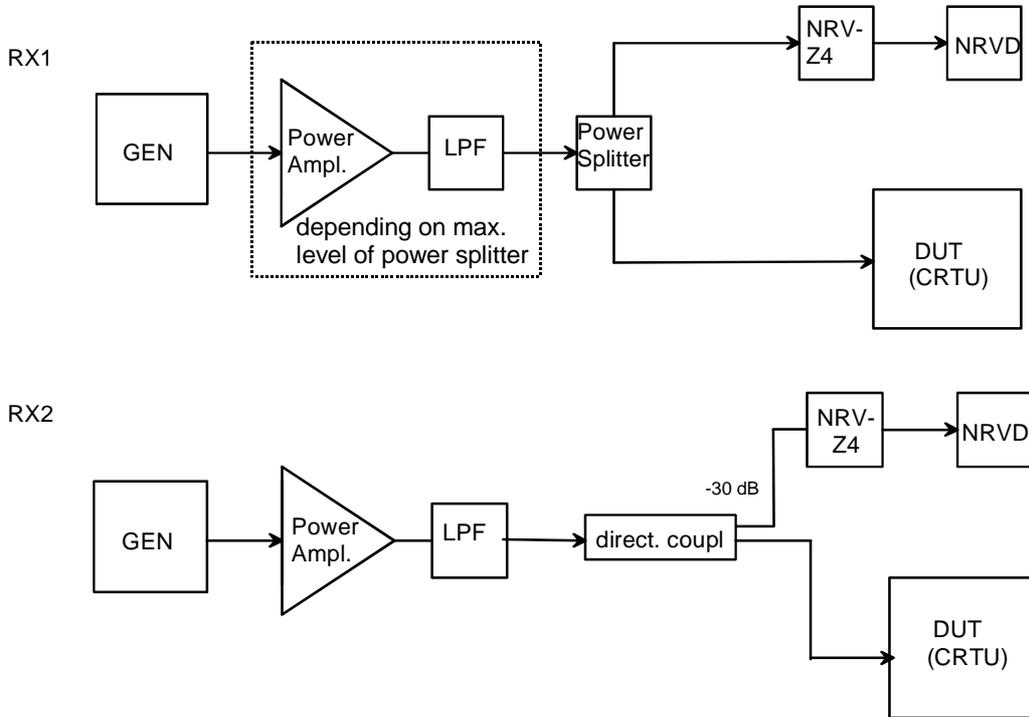
Fig. 1-4 Test setups for RX level measurements
