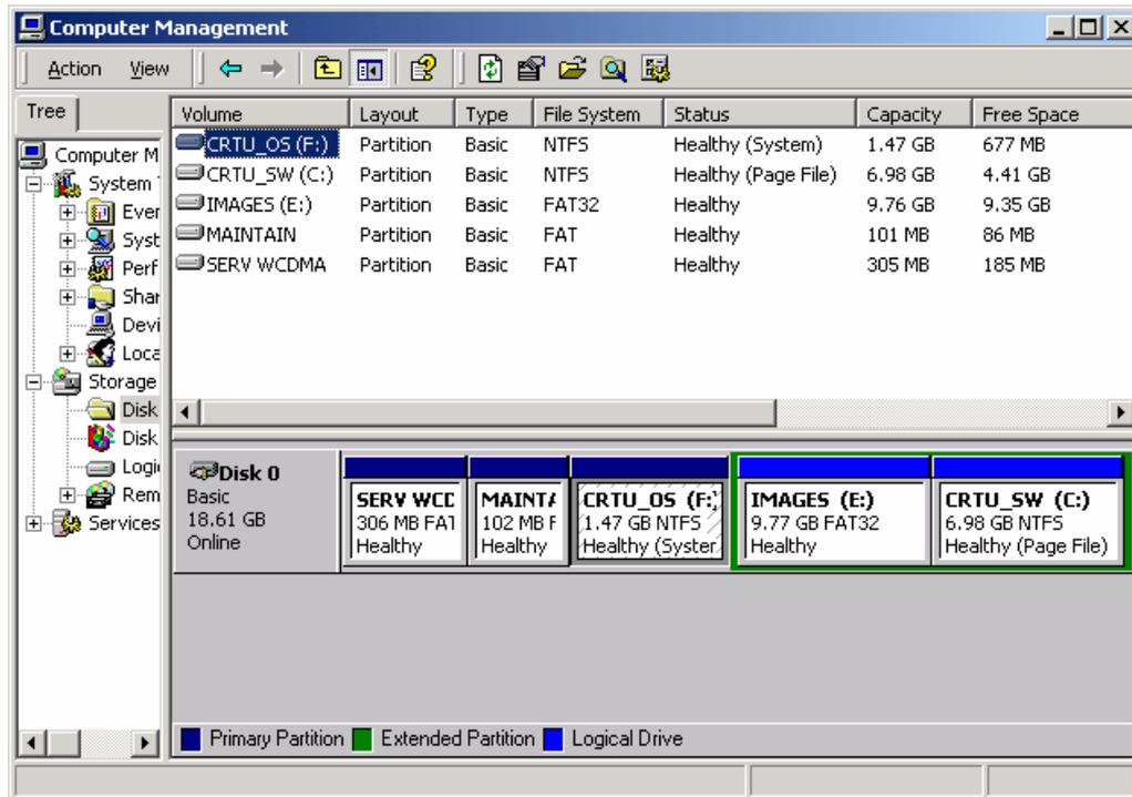
Fig. 4-2 Drive mapping after booting the GSM Operation Software (old partition structure)
