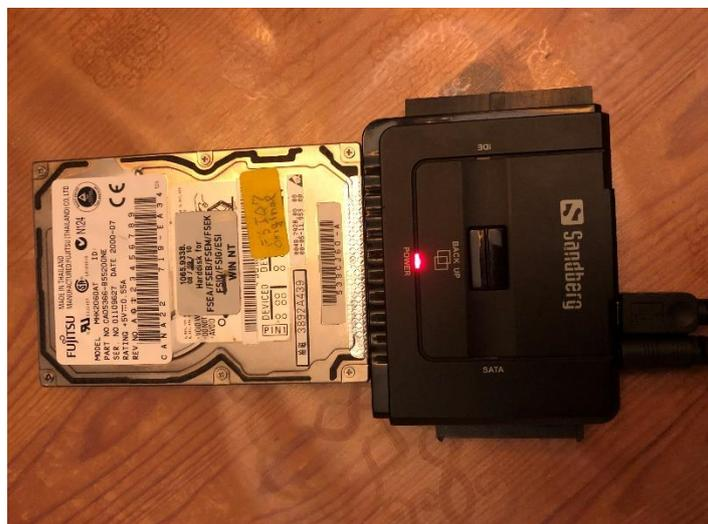
Plug the USB connector from the interface into an USB port. Both the content of the original HD which is named ROHDE is shown and by selection the Terminal Icon the screen look like this.
