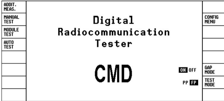
Press the TEST MODE softkey until FP is displayed in inverse video which indicates that the mode is active. Press the GAP MODE softkey until ON is displayed in inverse video and the GAP mode is active. Press the MANUAL TEST softkey. This opens the SIGNALLING FP-TEST menu where CMD60 searches for a dummy bearer signal ①.
