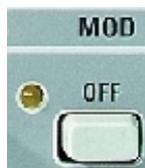
The different types of modulation can be switched directly by means of the [MOD ON/OFF] key or via the modulation menus. Modulation off is indicated by *OFF* in the status line in the **MODULATION** selection window and also by an LED.
