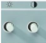
The screen contrast is adjusted by means of the right control knob (2), the brightness with the left control (1) below the display.
