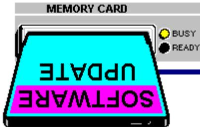
The MEMORY CARD with the program update is inserted into the front-panel slot and the appropriate menu is activated.
