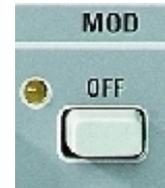
With the **MOD** OFF key all modulation signals of the currently used system are switched off:
