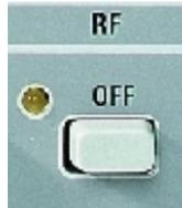
With the **RF** OFF key the RF output signal is switched off.
