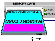
With the aid of the write-protection switch (1) the MEMORY CARD can be protected against inadvertent clearing. Fully insert the MEMORY CARD. In this position the green READY LED is on.
