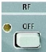
The RF output signal is switched on and off with the **RF ON / OFF** key. This has no effect on the current menu. When the output signal is switched off **RF OFF** is displayed in the **RF LEVEL** window. The off state is signalled in addition by an LED.
