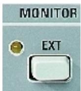
With the **MONITOR** EXT key the display is switched to the monitor output. At the same time the built-in LC display is blanked and the yellow MONITOR EXT LED lights.
