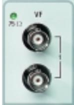
Connector VF (BNC) is a video input with a loopthrough filter. Either of the connectors can be used as an input or output. With an internal termination into 75  $\Omega$  the yellow LED lights. In this case the output of the loopthrough filter must not be terminated into 75  $\Omega$ .
